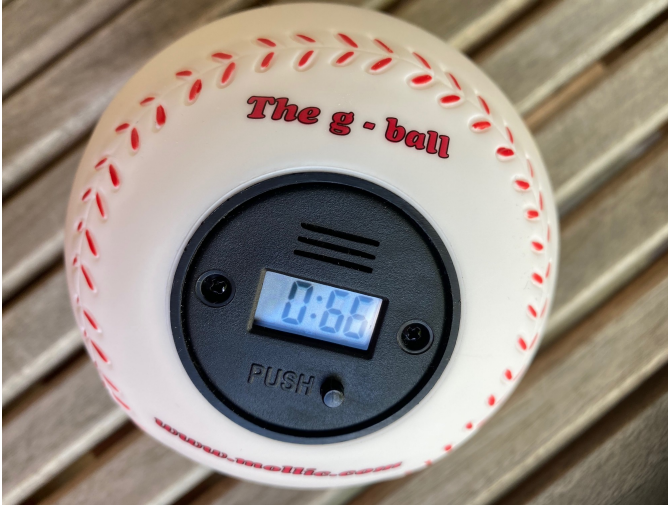
Fig. 1. The picture shows a ball with built-in stopwatch that starts when the ball is dropped (release of the button) and stops on impact. It has one-hundredth of a second precision. We have used this ball to indirectly measure the Planck length 100 times without knowledge of G or \hbar (as reported in Table 1.
