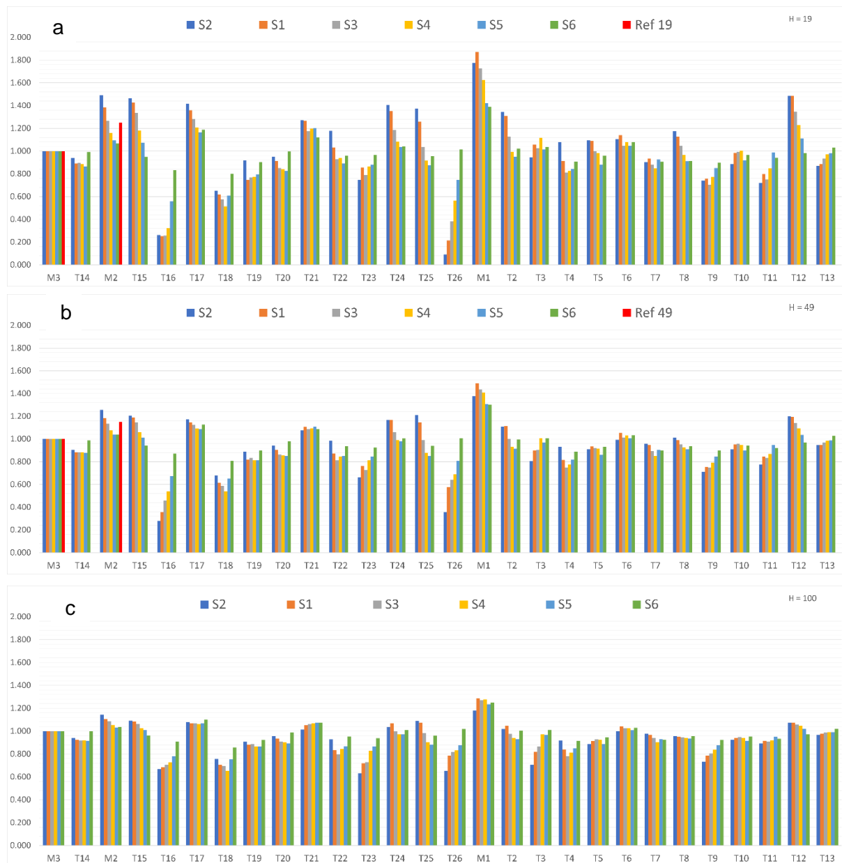
Figure 17 Normalized wind speed for all turbine positions in cases S2-S6. Displayed here for heights 19 (a), 49 (b) & 100m (c) above the terrain
