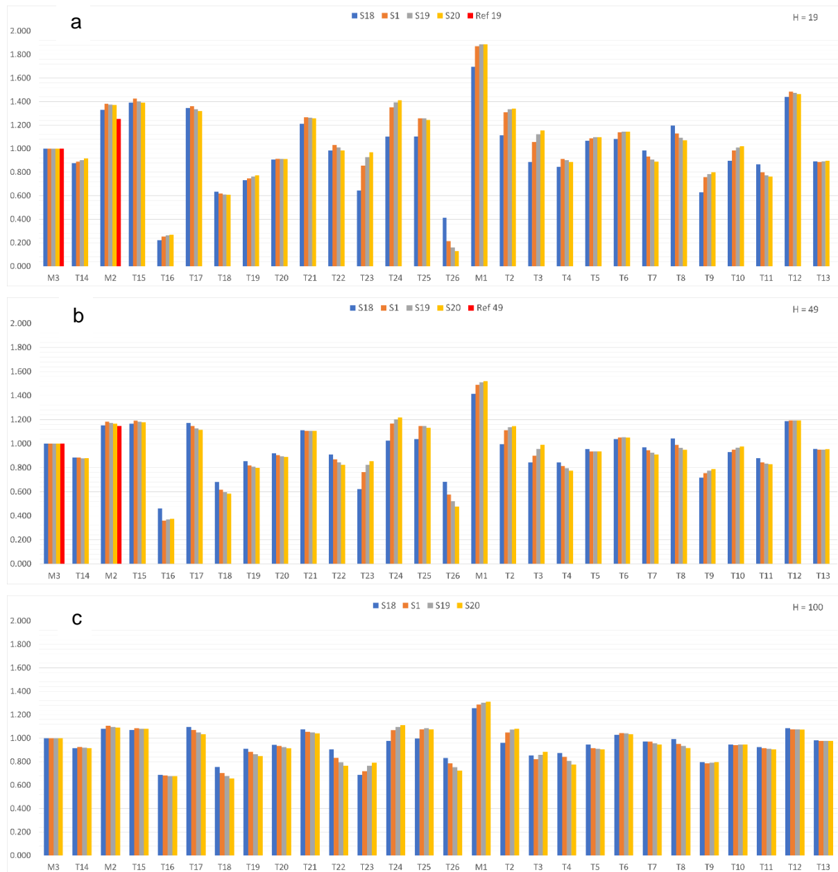
Figure 26 Normalized wind speed for all turbine positions in cases S18 - S20 at 19 (a), 49 (b) & 100m (c) above the terrain
