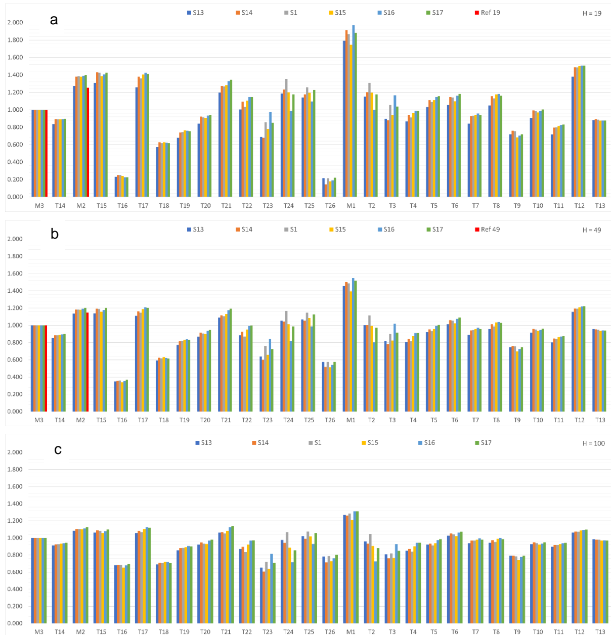
Figure 23 Normalized wind speed for all turbine positions in cases S13-S17. Displayed here for heights 19 (a), 49 (b) & 100m (c) above the terrain
