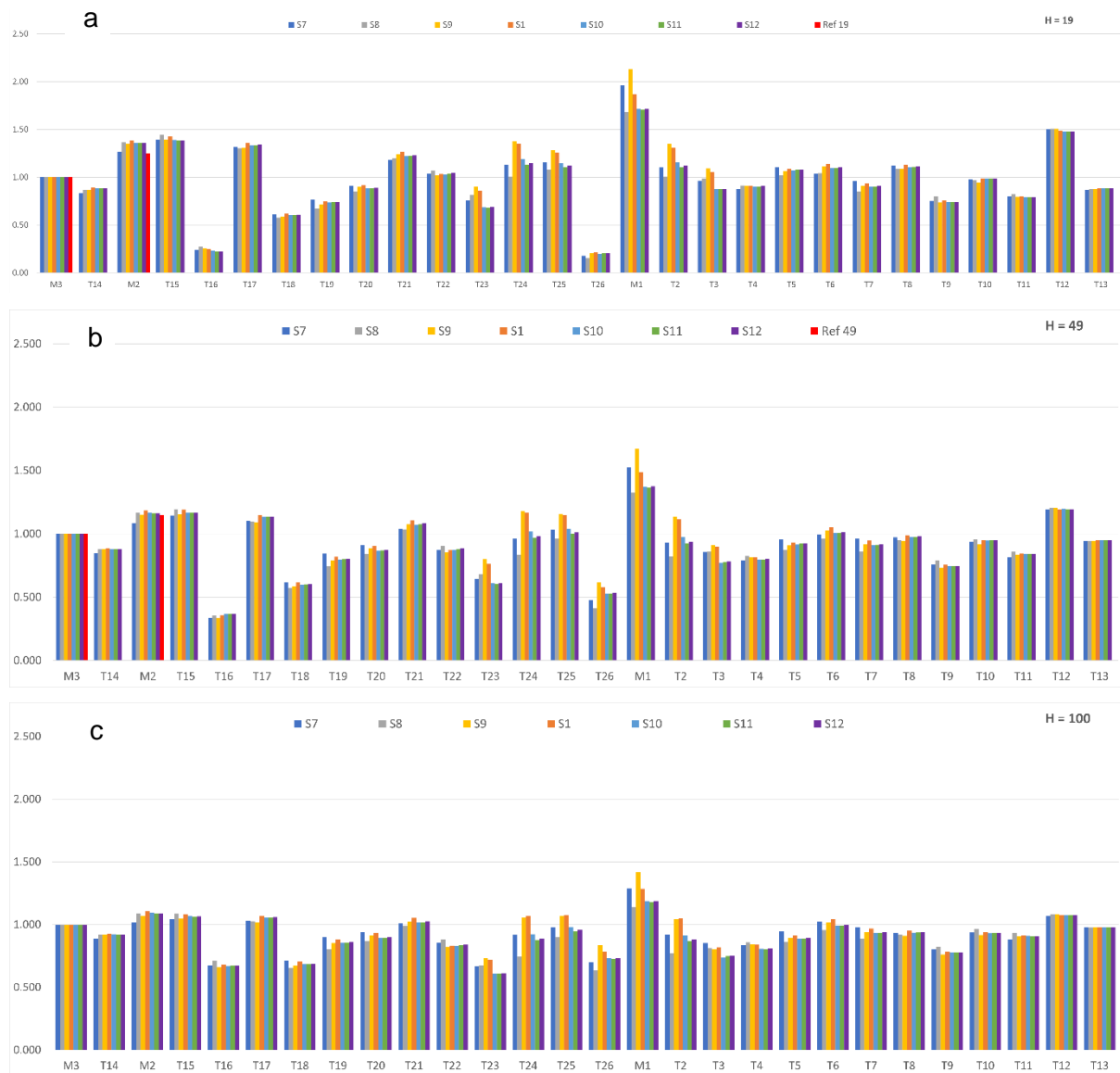
Figure 20 Normalized wind speed for all turbine positions in cases S7-S12 . Displayed here for heights 19 (a), 49 (b) & 100m (c) above the terrain.
