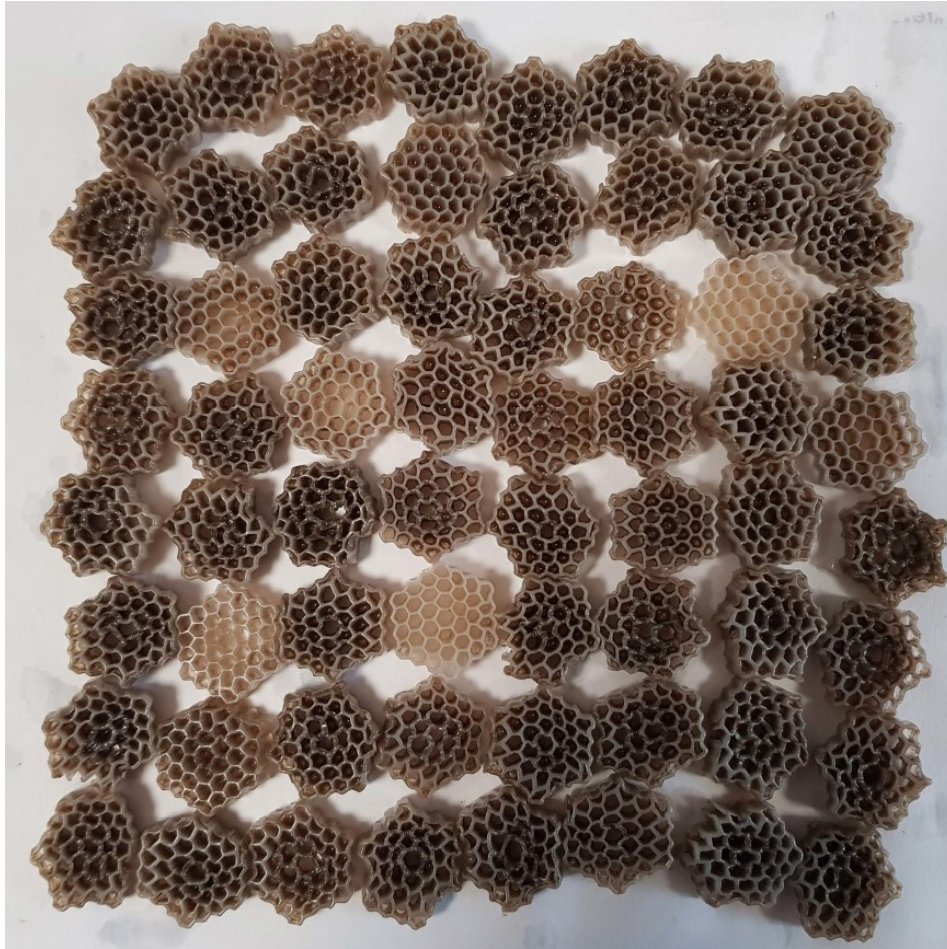
Figure 4.28: A representative selection of carriers from the SNR (two-reactor setup), showing some deformation.
