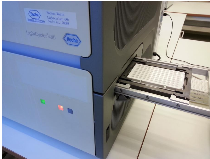
Fig. 14. LightCycler® 480 qPCR instrument and 96-well plate. By using this system, the change in fluorescence over the process of reaction is measured.
