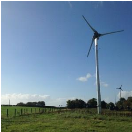
Figur 3.4 Kingspan Wind 15 KW. Kjelde: (Kingspan Wind 2015b).
