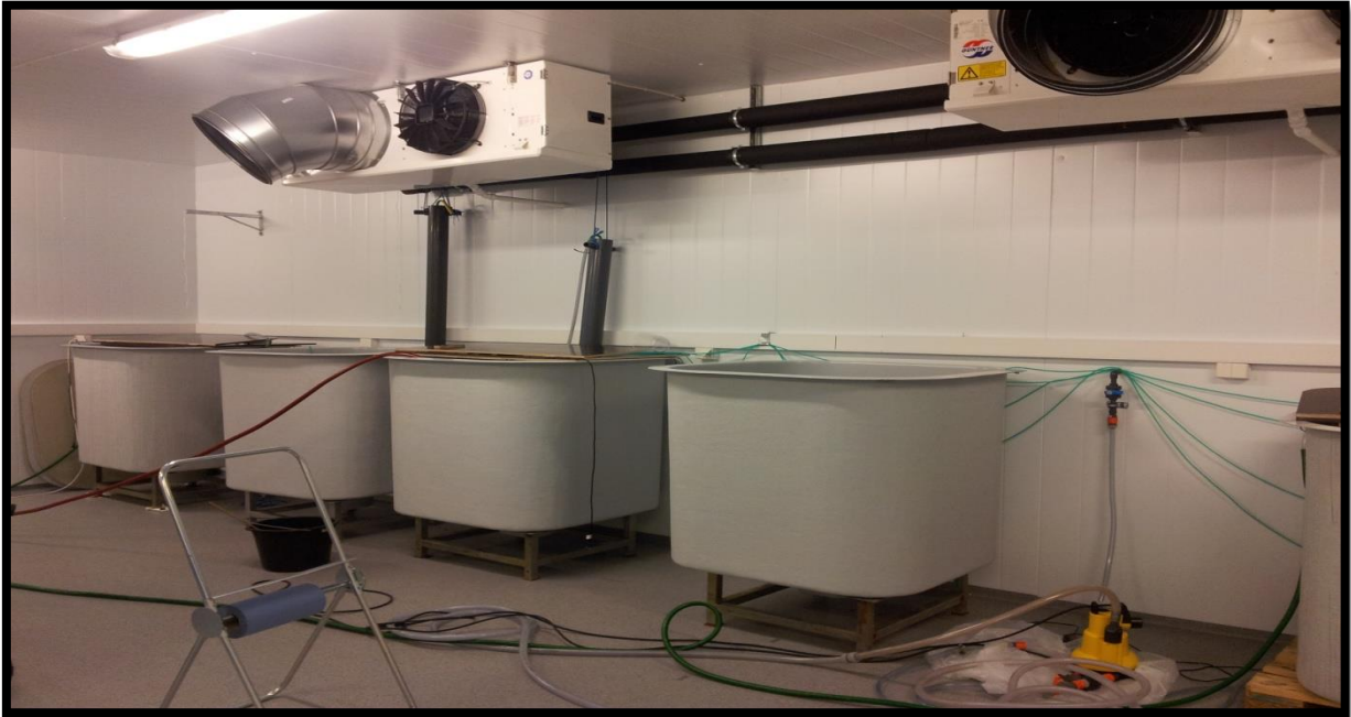
Figure 3. Glass fibre tanks with different water qualities used for acclimation of Atlantic salmon parr (Photo: Brice Sone).
