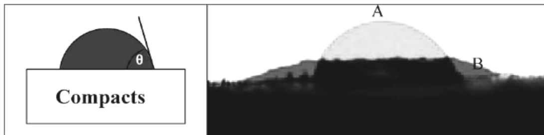
Figure 5.10. Typical example for the measurement of contact angle by the method sessile drop of compact (based on hard wheat flour). The initial contact angle (A) and after 3 min (B) (Roman-Gutierrez et al. 2003)
