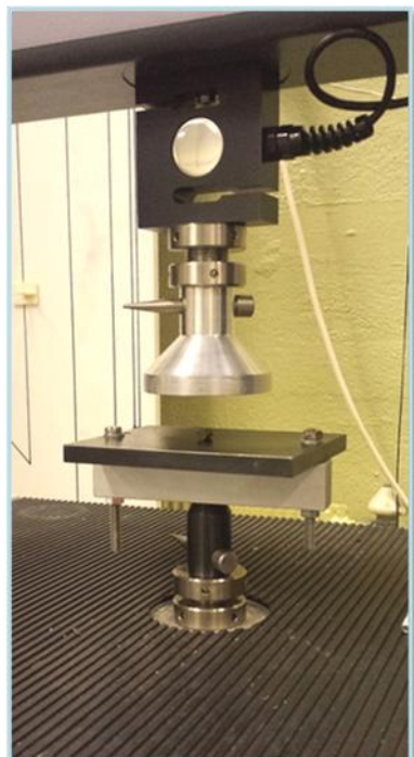
Figure 5.2. Diametric compression test connected to a Lloyd LR 5K texture analyzer
