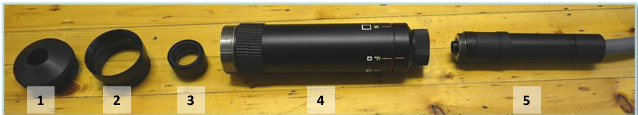
Figure 5.6. Assembling the video microscope. Items are indicated by numbers: (1) CVM Video probe head, (2) Zoom lens, (3) 20x – 120x basic lens, (4) Contact head adaptor, (5) 60x-420x contact head)
