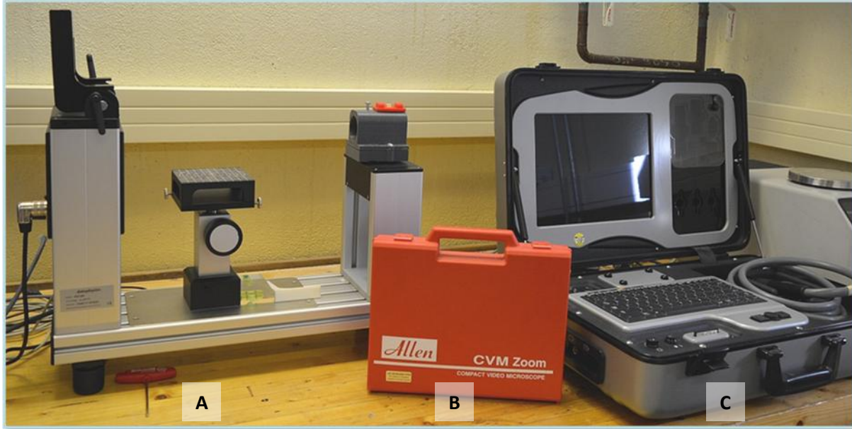
Figure 5.3. Equipment used for the evaluation of pellet water stability. Items are indicated by letters: (A) Krüss Tensiometer, (B) Allen Compact Video Microscope Lenses, (C) Micro Viper Portable Computer)
