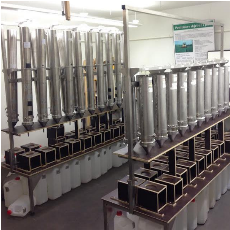
Figure 3. Column experiment setup in the lysimeter lab. (Photo source: Kristin Frøsland.)
