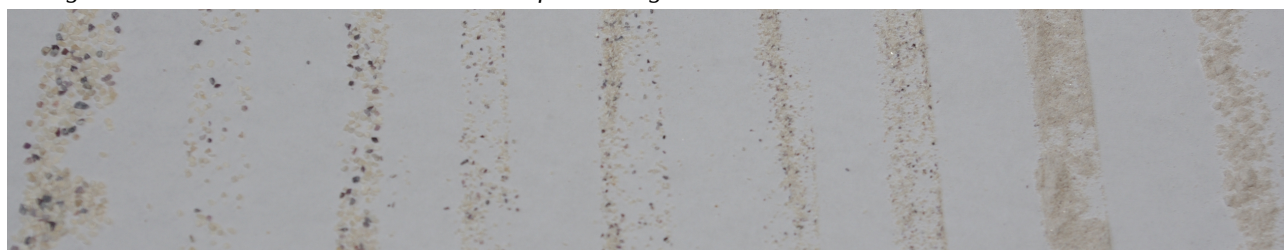
Figure 4.1.4: Fractions of sieved shell substrate, starting with sample 1 to the left and ending with sample 9 to right, table 4.1.1.
