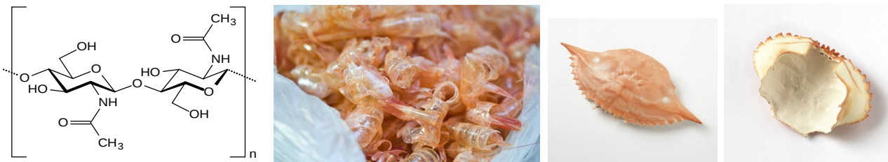
Figure 2.8: General structure of chitin [7] Fig. 2.9-2.11: Crustaceans shells from the seafood industry provides raw chitin [7]
