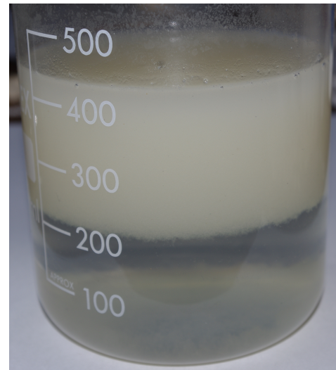
Figure 3.3.2d: flocculation, in this case the chitosan float as a result of air bubbles, after some stirring the chitosan phase will settle at the bottom.
