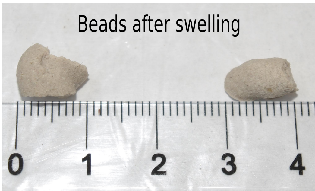
Figure 4.4.4: Beads with a high amount of cross-linking after swelling, the cross-linking was similar to sample 1, table 3.5.1.
