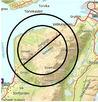
Figure 6.4: Cylinder model fit to the surface topography.
