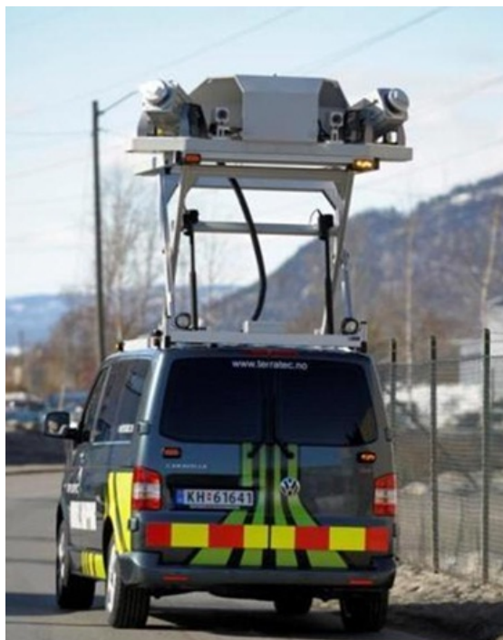
Figure 1.4: TerraTec Lynx Mobile Mapper exterior mounting of sensor instruments. The elevated ramp is about 4 m above ground. URL: http://www.terraTEC.no/ [2015-05-02]
