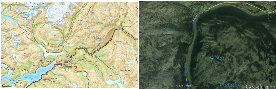
Figure 4.4: Overview and detail of the Lapplia tunnel. Screenshot from www.norgeskart.no (left) and Google Earth (right) [Downloaded 2015-04-03]. KML overlay of post-processed trajectory exported from the TerraPos solution.
