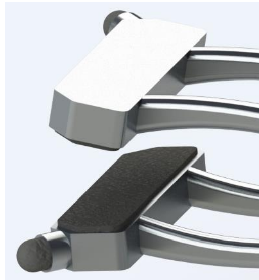
Figure 12.2: Design of the gripper with touch tips
