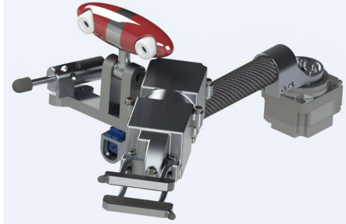
Figure 12.11: Tool, vibration sensor and camera added to last link of arm.
