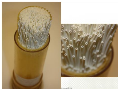
Figure 3: Shows a hollow fiber membrane. Diffusion occurs along the tube side of the many white pipes. Obtained from lecture notes in TMPP 100.
