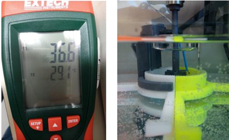
Figure 38: The picture to the left shows T1 and T2 where T1 is for the stomach and T2 for the water bath. The picture to the right shows the temperature sensor (blue wire in the stomach).
