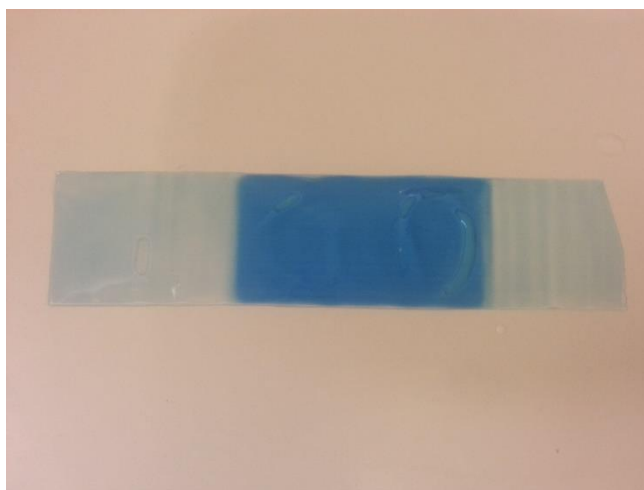
Figure 25: This picture shows that the color of Evan's blue is difficult to wash away. This is an indicator of fouling.
