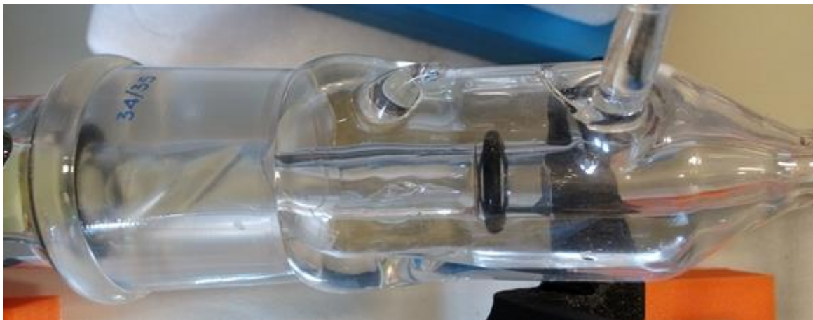
Figure 35: This figure shows the membrane collapse in a small test for functionality. Inside and outside the membrane water flows.
