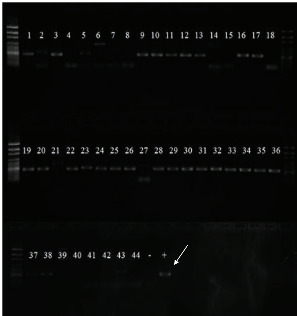
Figure A.4 Gel electrophoresis of the int1 PCR products for the possible int1 positive samples. A negative control (-) and a positive ( E. coli ) control (+) were included. The positive control shows the int1 fragment (~530 bp) highlighted by the arrow. The contrast is increased for better visualization of the fragments.
