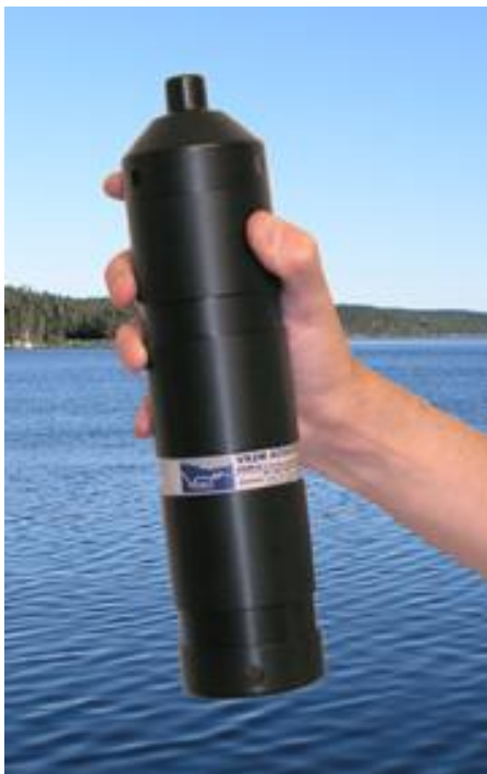
Figure 6: A VR2w receiver for passive monitoring of tagged sea trout (Photo credit: www.Vemco.com )
