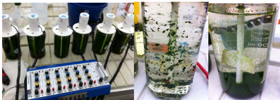
Figure 26 - Jar Test apparatus, by Kemira, Finland, with six beakers of 1L in process of mixing algae suspension with pipetted flocculant dosage (left). Flocs still in movement after stirring with stirring paddle (center). Settled flocs and the bottom of the beaker of 1L treated microalgae, and the water phase (right).
