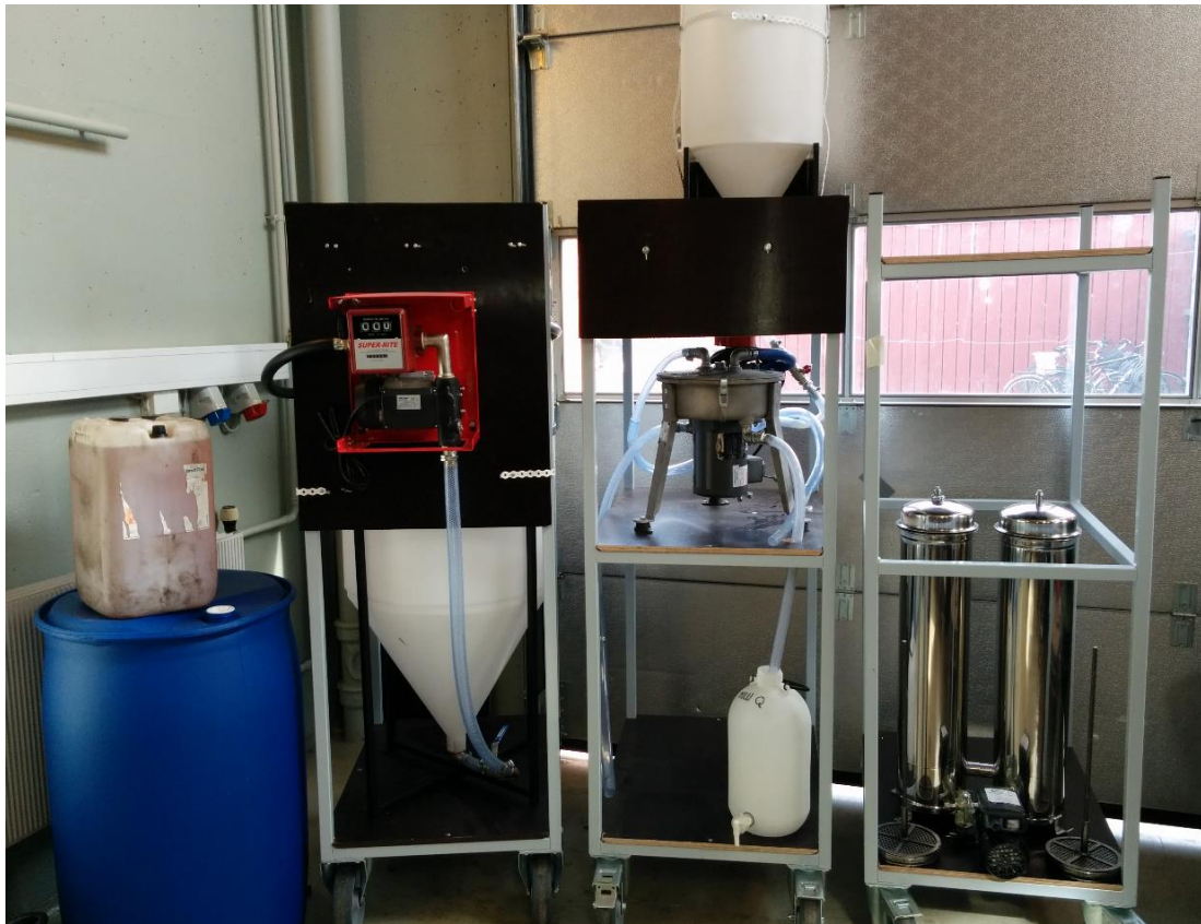
Figure 4.19: The part of the plant constructed (from left to right): HDPE barrel with a tank of WCO on top of it, mixer, separator with a 60 L conic tank above it and the reactor rig.
