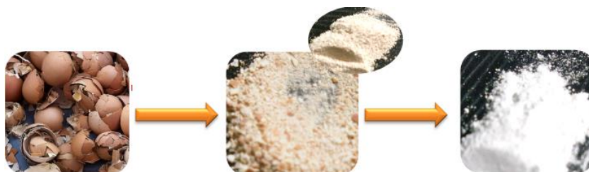
Figure 3.2: Eggshell are crushed into a powder and then calcinated to CaO [37].
