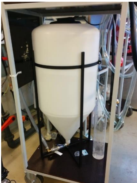
Figure 4.11: 200 liter conical tank and mixer [67].
