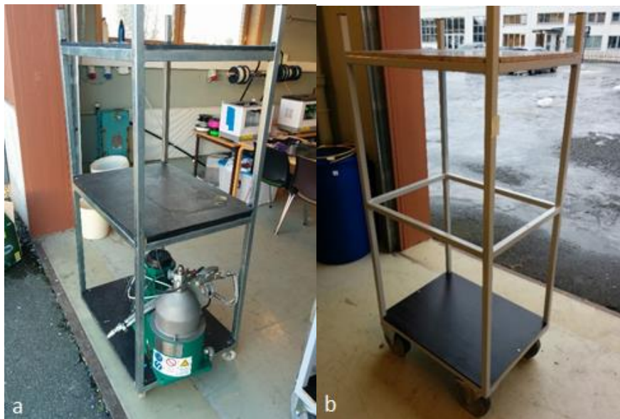
Figure 4.1: The framework prototype (a) with a centrifuge and the new framework (b).
