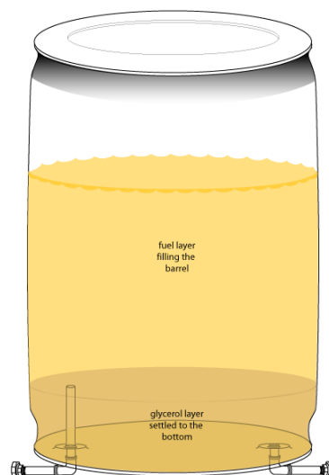
Figure 2.9: Separation of glycerol (bottom) and biodiesel (upper) in a settling tank [26].
