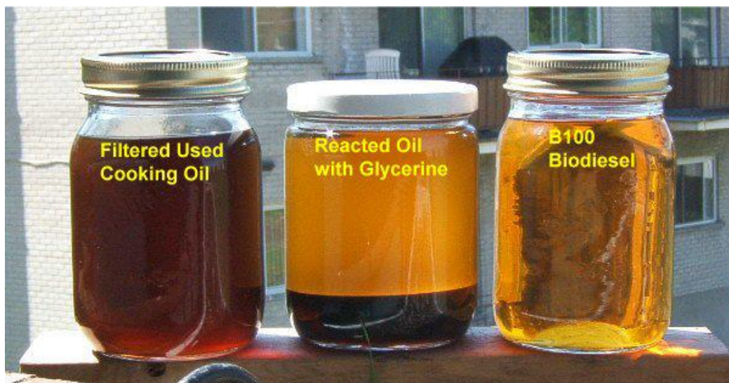
Figure 2.5: Esterification of used cooking oil with sulfuric acid illustrated [14].
