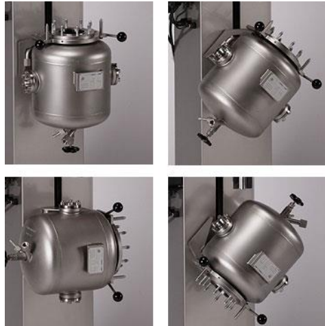
Figure 4.8: A reactor with a tilt-mechanism [63].
