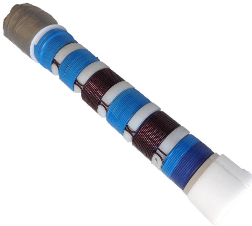
Figure 8.1: Assembled stator, with winding spacers, endcap winding spacers and windings installed. Some windings are left unprotected for illustration purposes.
