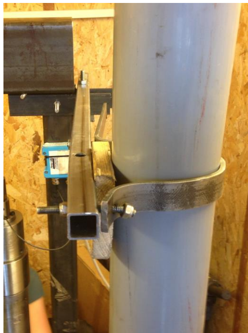
Figure 8.6: Rigging of the post driving test, with custom clamps.
