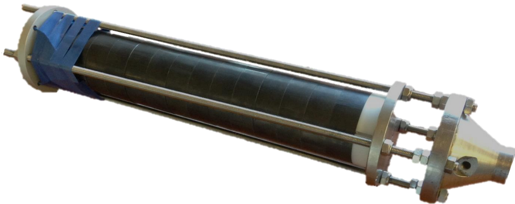
Figure 8.3: Picture showing the finished assembly of stator with SMC rings, piston, end caps and striking head. Wires are taped over for protection.
