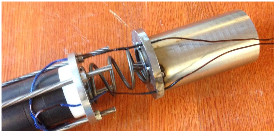
Figure 8.2: Picture of the spring welded between the stator and the top end with mass.
