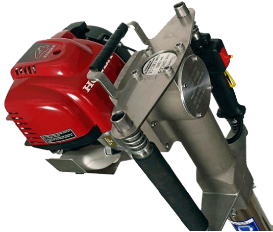
Figure 1.2: Petrol engine from honda mounted on a post driver. Source: http://www.petrolpostdriver.com/
