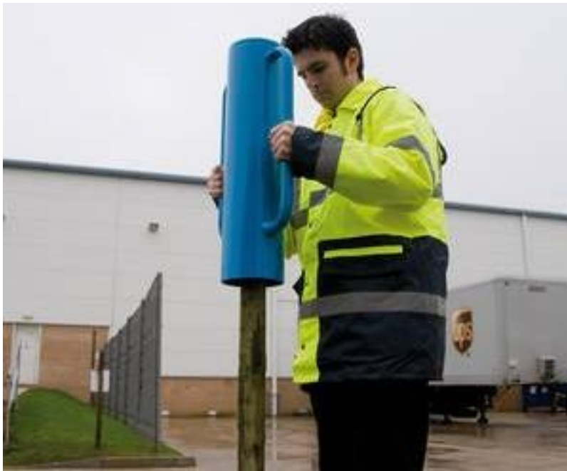
Figure 1.1: Manual post driver being used to drive a wooden post. Source: http://www.gustavsenas.no/
