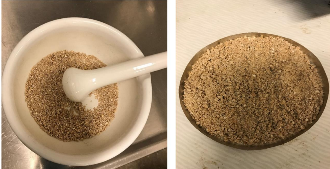
Figure 5. The mortar and the pestle used to grind pellets were shown on the left side. And the metal tray with ground materials was presented on the right side.
