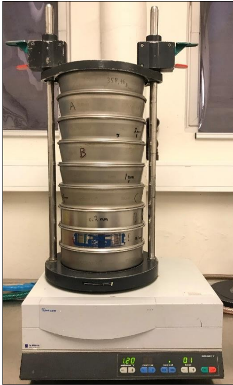
Figure 6. A presentation of the dry sieving assembly.
