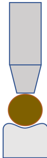
Figure 3. A schematic figure of the functional zone of a Kahl hardness tester (Inspired by Lowe (2005)).
