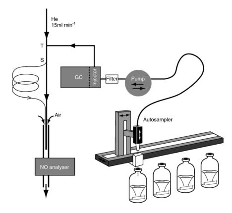
**Figure 3. 2. The robotized incubation system designed by Molstad et al. (2007).** The gases are sampled from vials using a peristaltic pump with He as the carrier gas and transported to a gas chromatograph (GC) and an NOx analyzer to analyze the headspace gas composition at different time points.
