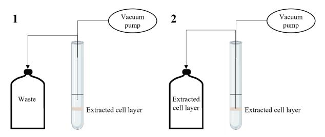
Figure 3. 3. Setup for siphoning off the extracted bacterial cell layer on top of the Nycodenz layer. 1) A vacuum pump was used to remove the supernatant above the extracted cell layer before 2) the extracted cell layer was vacuumed off into a fresh vial.
