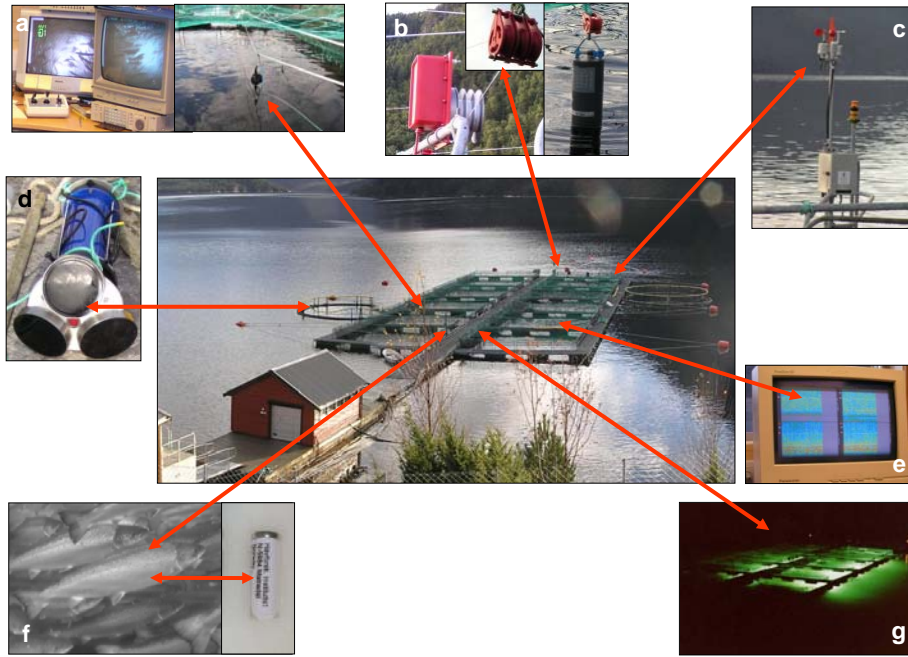
Figure 9 Pictures and sketch of the cage environment laboratory at IMR. a) Remote control cameras observe individual and group behaviour, b) CTD's attached to automatic winches records depth profiles of temperature, salinity, dissolved oxygen and light, c) A weather station measures wind and air temperature, d) Acoustic current profilers measures water current speed and direction around the cages while a velocimeter is used inside cages, e) A PC based echo sounder records the swimming depth and fish density of groups, f) Data Storage Tags records swimming depth and thermal history of individual fish, and g) Underwater lamps can be deployed at different depths. Photo: IMR.
