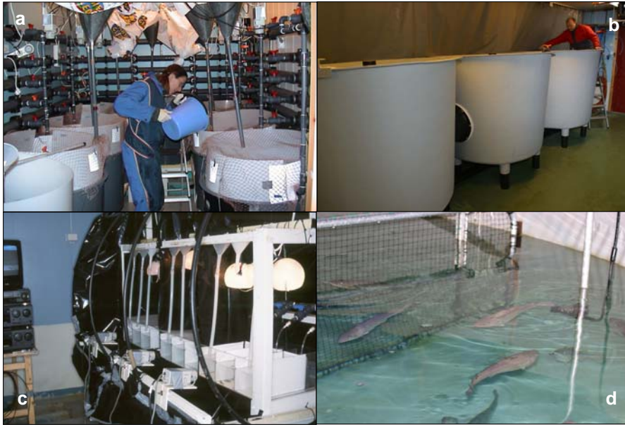
Figure 2 Tank units for observation of fish behaviour at Fiskeriforskning. a) Regular 100 l rearing tanks with video cameras above each tank, b) 1700 l preference tanks with PIT-tag antennas in the channel between each tank and video cameras above each tank, c) 6 l aquariums for juvenil fish with cameras on the side of the aquariums, and d) 5-m diameter large scale tank with underwater pole camera and zoom cameras above the tank. Photo: Fiskeriforskning.
