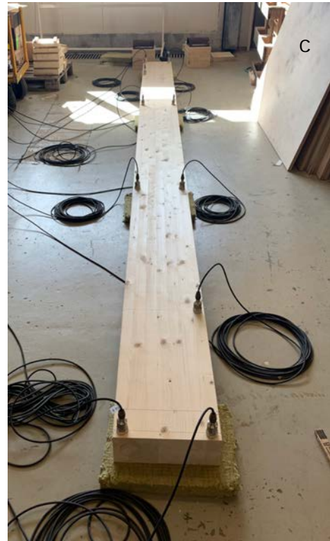
Fig. 4. a) Test setup glulam beams, b) Test setup plywood boards, c) Test setup for torsional modes glulam beams. (all the dimensions are in mm)
