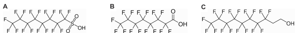
Figure 3. An overview of different classes of PFCs. Carbon chain in PFCs can bind to A) sulfonic acids (PFOS), B) carboxylic acids (PFOA) and C) fluorotelomer alcohol (FTOH). Figure was adapted from [32].
