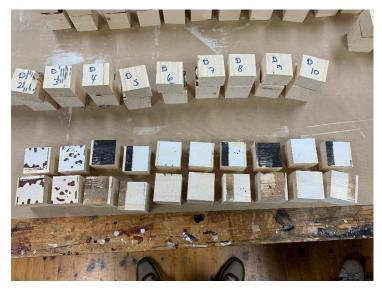
Figure 26: Glue line fractures, Painted-100g-glue
