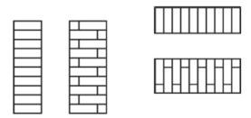
Figure 6: Glued laminated timber, figure 4 from NS-EN 14080
