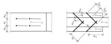
Fig. 4. Definition of spacings, end and edge distances for axially loaded screws.
