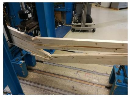
Figure 23: Combination of shear and bending fracture
