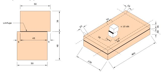
Figure 20: Preparation of glue line test bars, Illustration: Andreas Stenstad, NTI
