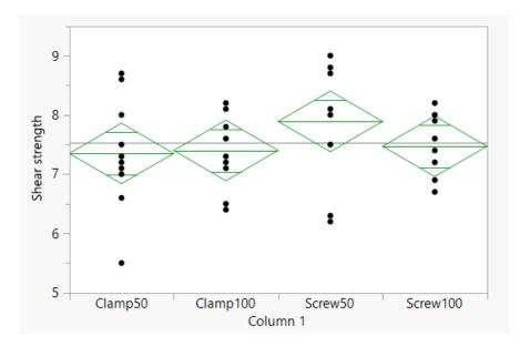
Figure 29: Analysis of variance, Shear strength by type, clamp- and screw-samples
