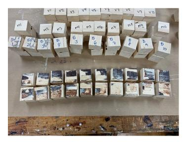
Figure 33: Glue line fractures, Clamps-50g-glue
