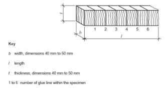
Figure 8: Test bar and numbering of the glue lines, figure D.2 from NS-EN 14080
