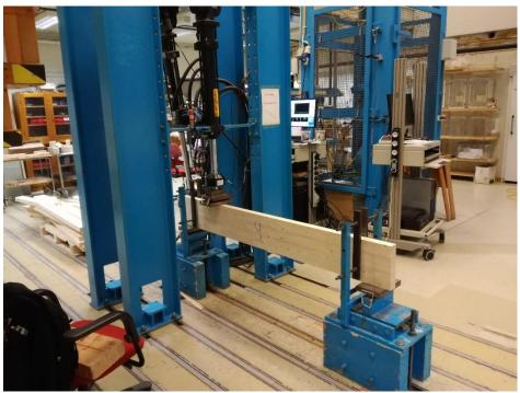
Figure 15: Test setup for beams
