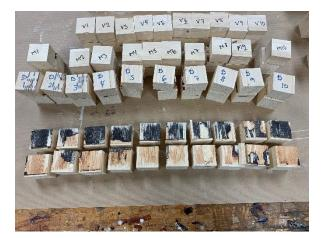
Figure 37: Glue line fracture, Wet-200g-glue
