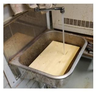
Figure 16: Preparation of wet samples
