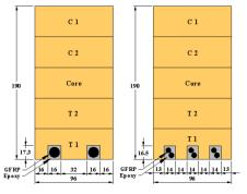
Figure 1: Reinforcement arrangement for repaired 190mm deep beams.
