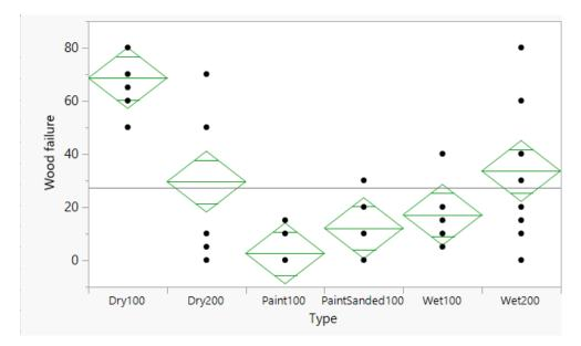
Figure 32: Analysis of variance, Wood failure, Self-weight samples
