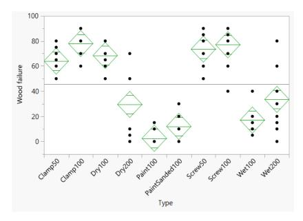
Figure 28: Analysis of variance, Wood failure by type
