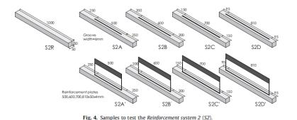
Figure 12: Morales-Conde (2015). Samples to test the Reinforcement system 2 (S2). In: Morales-Conde, M. J., Rodríguez-Liñán, C. & Rubio-de Hita, P. (2015). Bending and shear reinforcements for timber beams using GFRP plates. Construction & building materials, 96: 461-472. doi: 10.1016/j.conbuildmat.2015.07.079.
