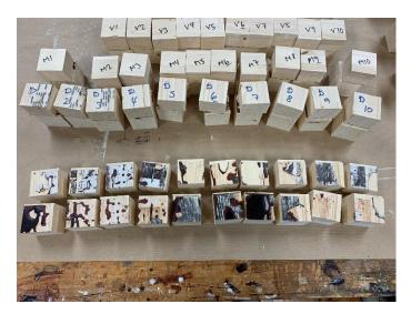
Figure 38: Glue line fracture, painted ad sanded down
