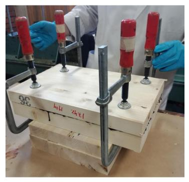
Figure 19: Glue line sample with clamps
