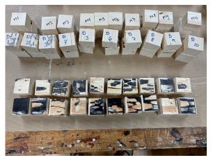
Figure 36: Glue line fracture, Wet-100g-glue
