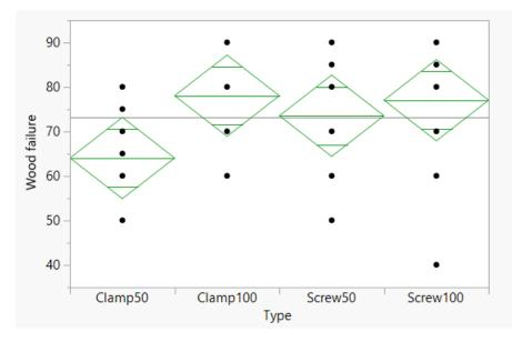
Figure 30: Analysis of variance, Wood failure by type, clamp- and screw-samples
