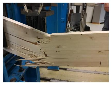
Figure 22: Bending fracture of beam
