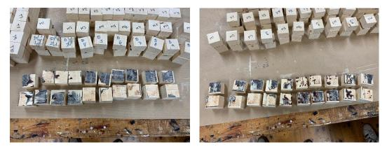
Figure 35: Glue line fracture, dry-200g-glue
