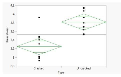
Figure 24: Analysis of variance, cracked and uncracked beams
