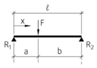
Figure 13: Asymmetrically placed load, SINTEF Byggforsk 421.051
