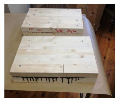
Figure 18: Glue line sample with screws
