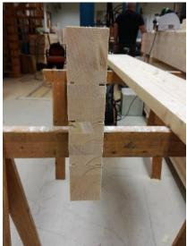
Figure 14: Sawn-in cracks
