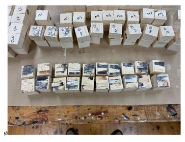
Figure 25: Glue line fractures, Screws-50g-glue
