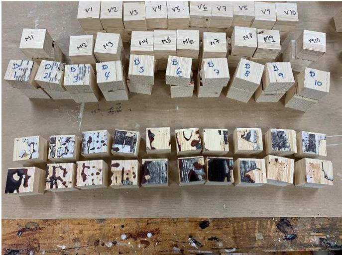
Figure 38: Glue line fracture, painted ad sanded down
