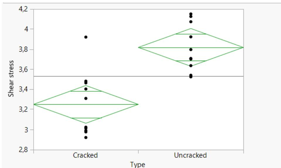
Figure 24: Analysis of variance, cracked and uncracked beams
