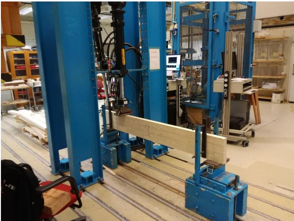
Figure 15: Test setup for beams
