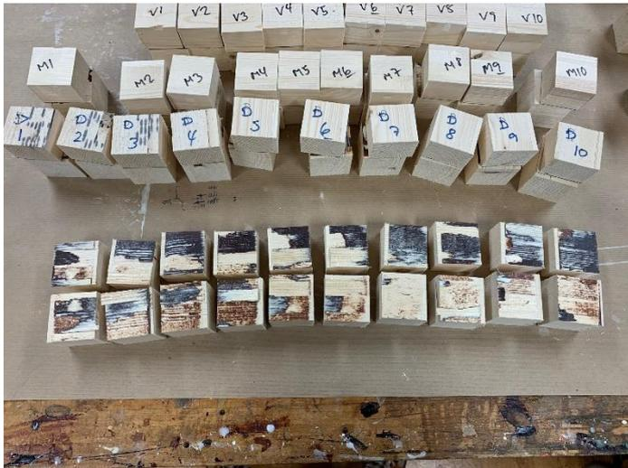
Figure 33: Glue line fractures, Clamps-50g-glue
