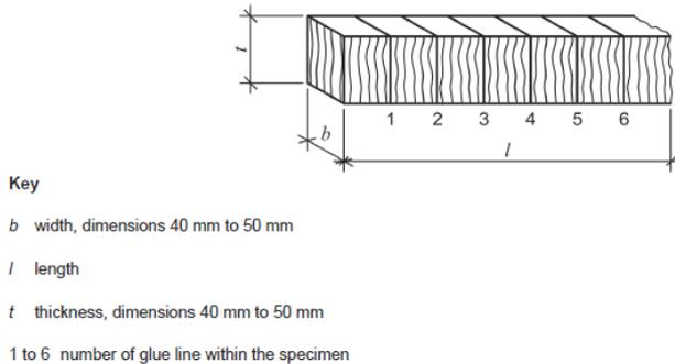
Figure 8: Test bar and numbering of the glue lines, figure D.2 from NS-EN 14080
