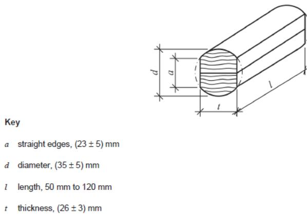
Figure 9: Drill core with machine parallel plane surfaces, figure D.3 from NS-EN 14080
