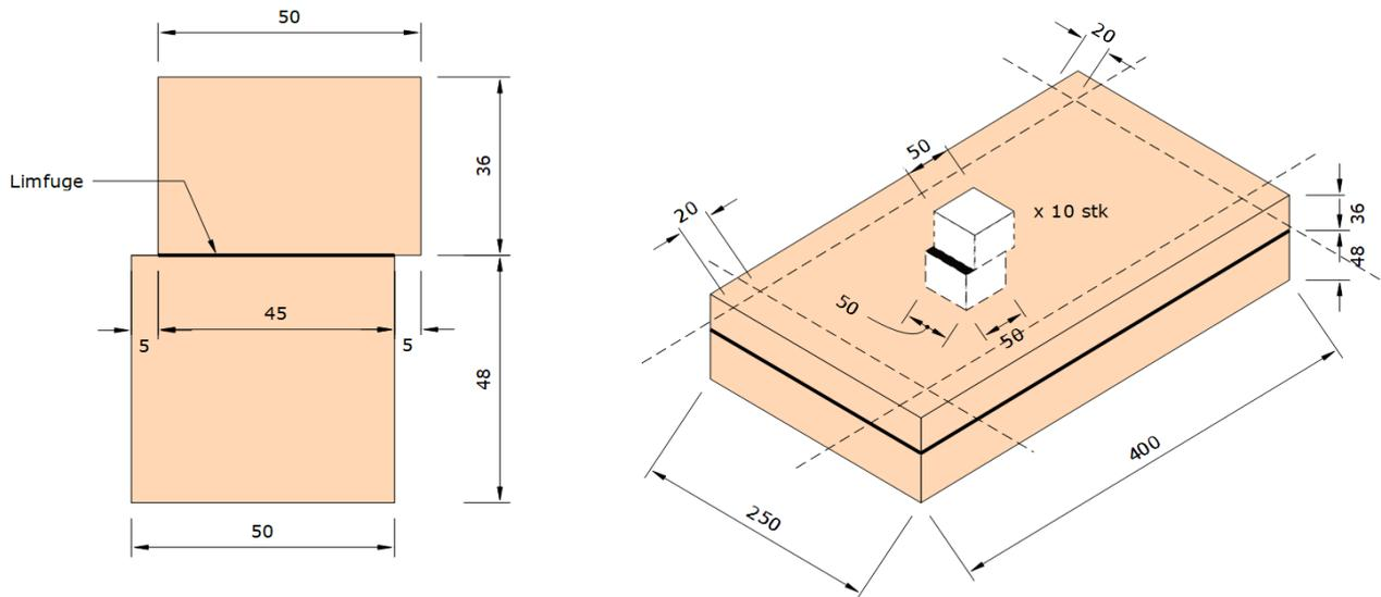
Figure 20: Preparation of glue line test bars, Illustration: Andreas Stenstad, NTI
