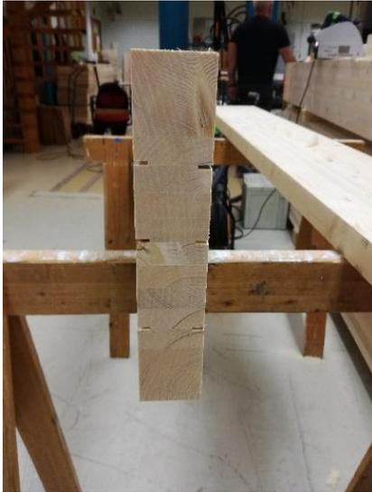
Figure 14: Sawn-in cracks
