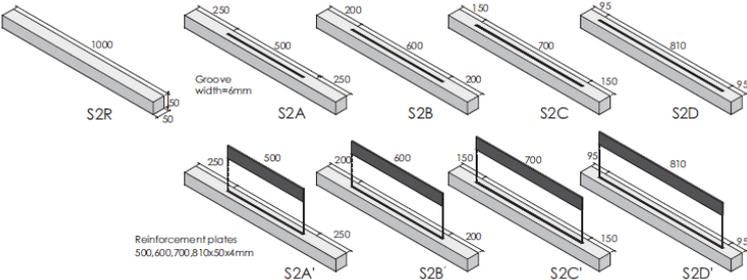
Fig. 4. Samples to test the Reinforcement system 2 (S2).
