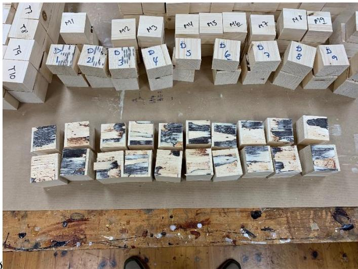
Figure 25: Glue line fractures, Screws-50g-glue
