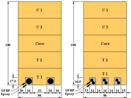
Figure 1: Reinforcement arrangement for repaired 190mm deep beams.
