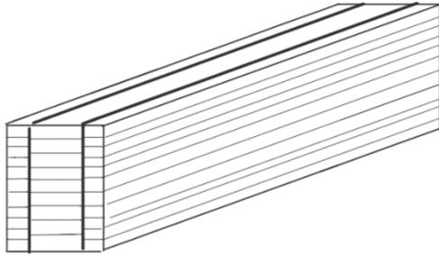
*Figure 5: Repaired glulam beam*
