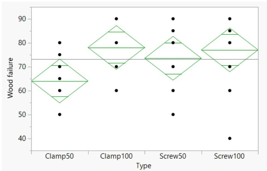
Figure 30: Analysis of variance, Wood failure by type, clamp- and screw-samples
