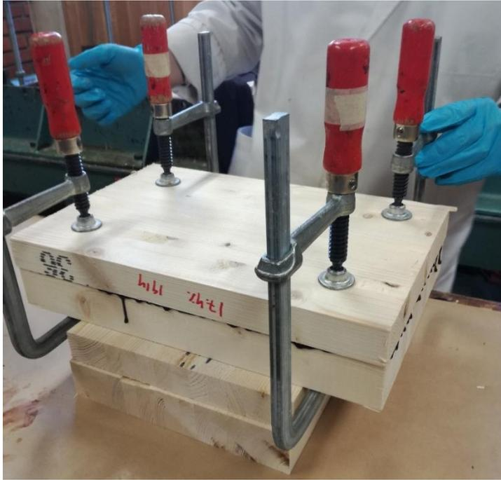
Figure 19: Glue line sample with clamps
