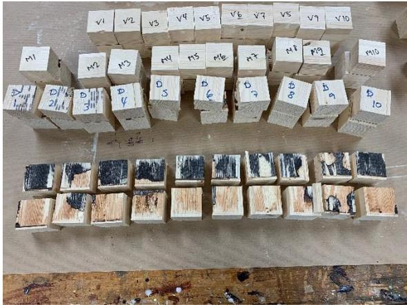
Figure 37: Glue line fracture, Wet-200g-glue
