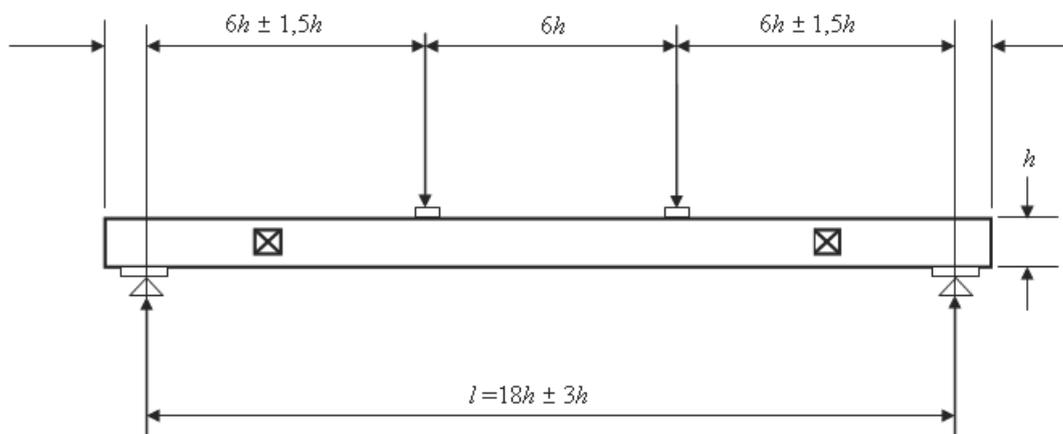
Figure 7: Test arrangement for shear field test, figure 7 from NS-EN 408
