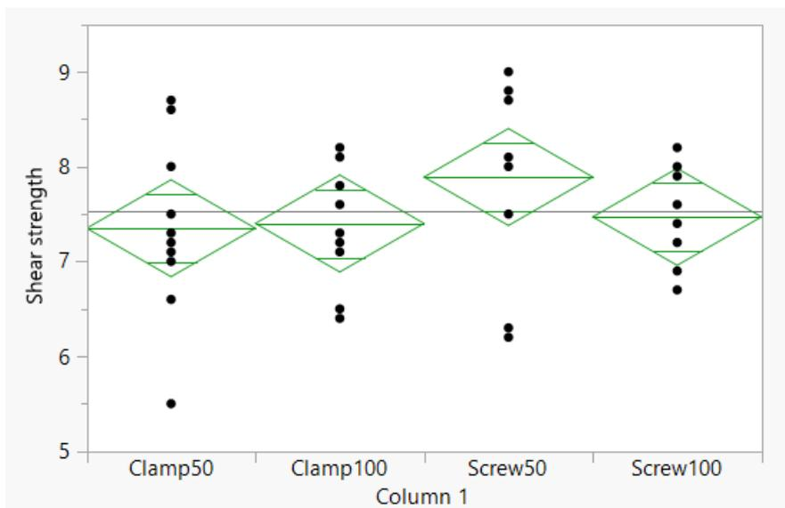
Figure 29: Analysis of variance, Shear strength by type, clamp- and screw-samples
