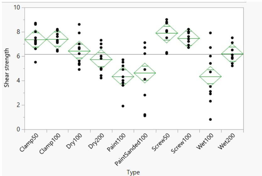
Figure 27: Analysis of variance, Shear strength by type
