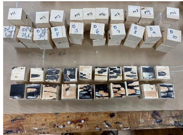
Figure 36: Glue line fracture, Wet-100g-glue
