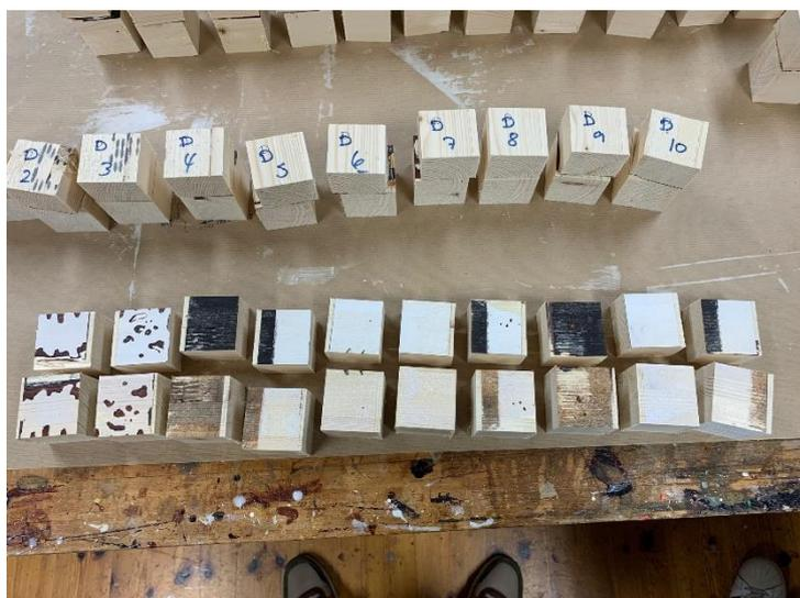
Figure 26: Glue line fractures, Painted-100g-glue
