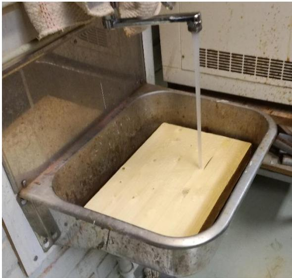
Figure 16: Preparation of wet samples
