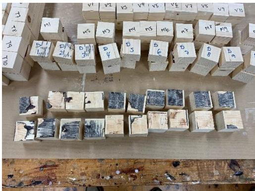
Figure 35: Glue line fracture, dry-200g-glue
