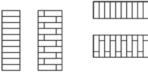
Figure 6: Glued laminated timber, figure 4 from NS-EN 14080
