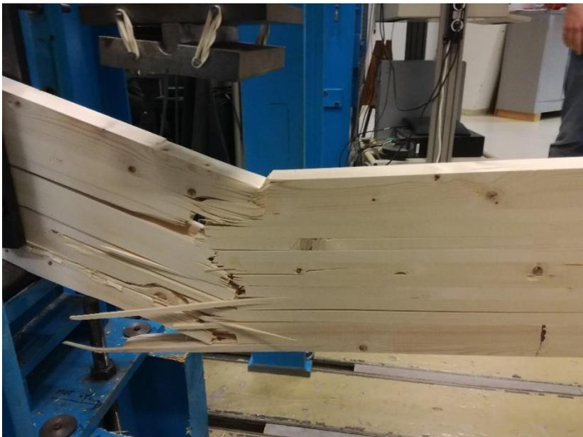
*Figure 22: Bending fracture of beam*
