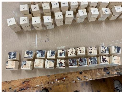
Figure 34: Glue line fracture, dry-100g-glue
