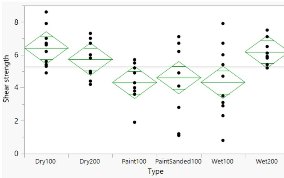
Figure 31: Analysis of variance, Shear strength, Self-weight samples
