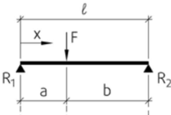
Figure 13: Asymmetrically placed load, SINTEF Byggforsk 421.051
