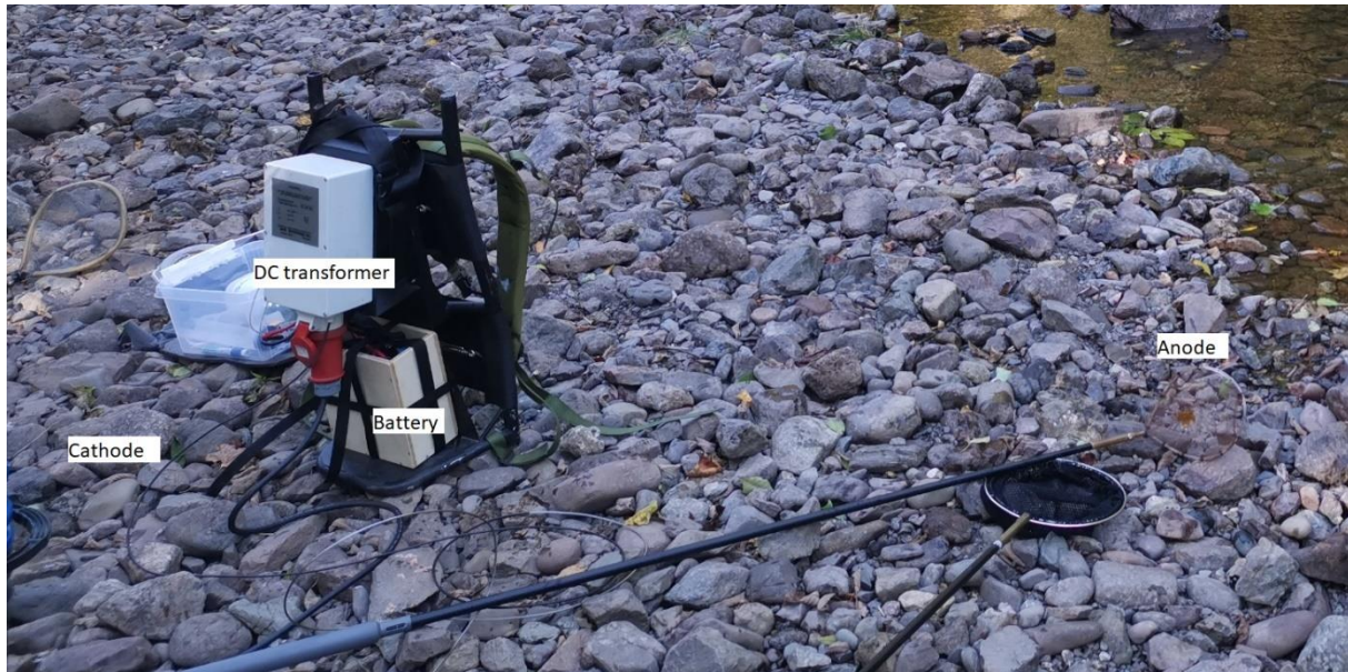
Figure 7: Electro-sampling gear consisting of a DC transformer, a battery, a cathode and a hand held anode. The transformer and the battery are rigged onto a backpack and the cathode trails downstream in the river while in use.
