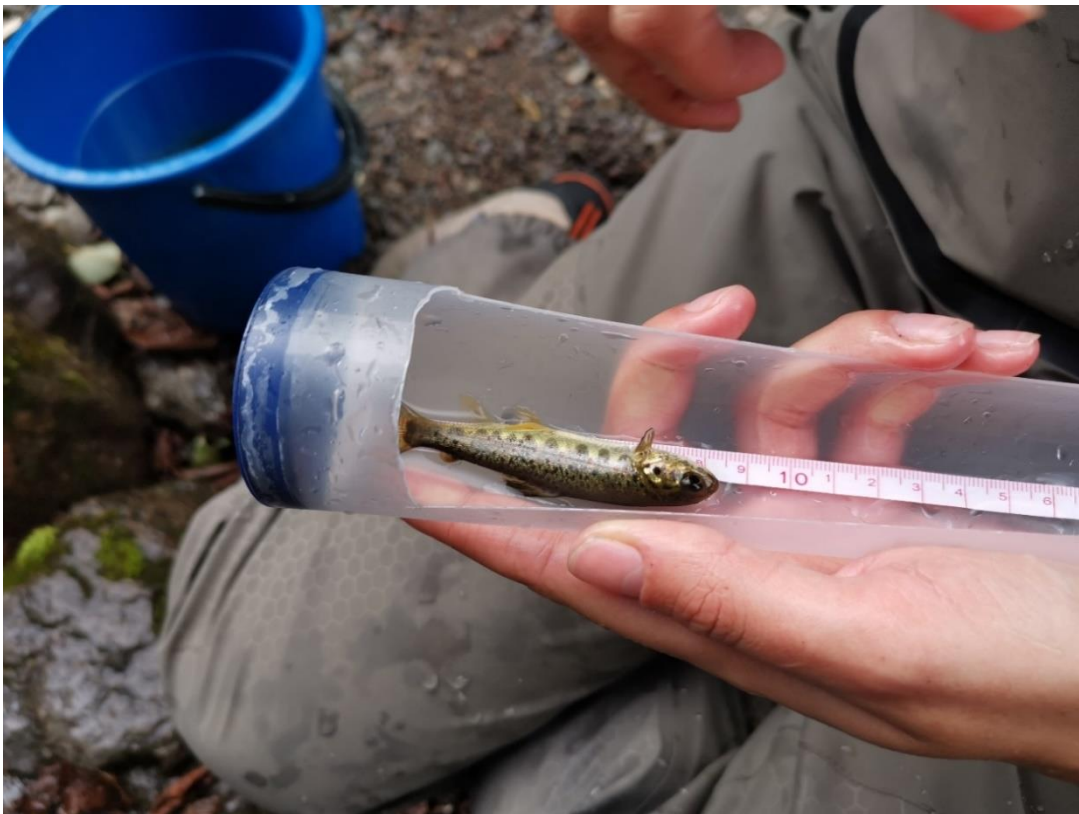
Figure 10: Length was determined using a measuring tape glued to half a cylinder. Here a salmon parr is measured in ISI1 station.
