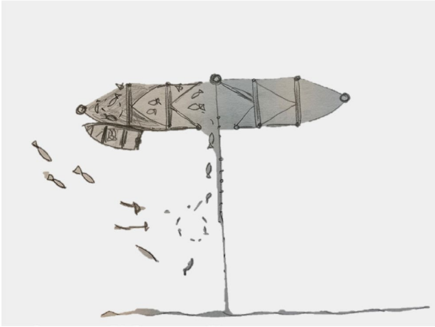
FIGURE 2 Double bagnet (kilenot). Fixed gears seen from above. Tied up to land with a net who leads salmon in to the “fish rooms” in the ends of the net. Salmon swim through wedges into the “big room” and further into the “fish room” where they normally are caught alive
