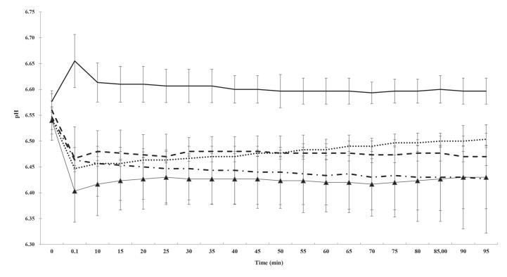
Figure 2. Change in pH during the diafiltration process of microfiltration retentate. – reference; – · – lactic acid; – – HCl; –  $\blacktriangle$  – citric acid; · · · · carbonated water. Means ± SD.
