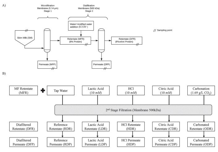
Figure 1. Schematic representation of (A) 2-stage filtration process of microfiltration (MF) and diafiltration (DF) and (B) details of DF treatments and nomination. DV = diavolume.
