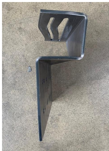
Figure 7-23 Deformed shape of STD-2H in test 19
