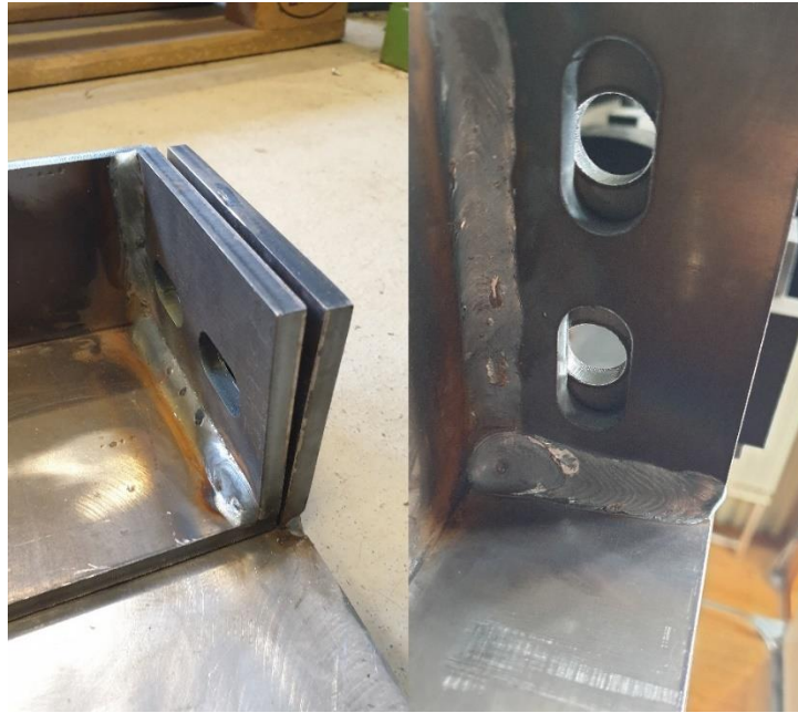
Figure 7-18 Imperfection in the ALT-AS specimen
