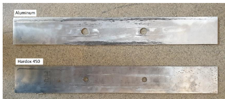
Figure 7-26 Damage to the aluminum and Hardox 450 shim layer
