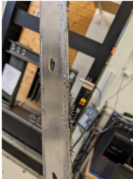
Figure 7-30 Magnetic Hardox steel residue on ALT M20
