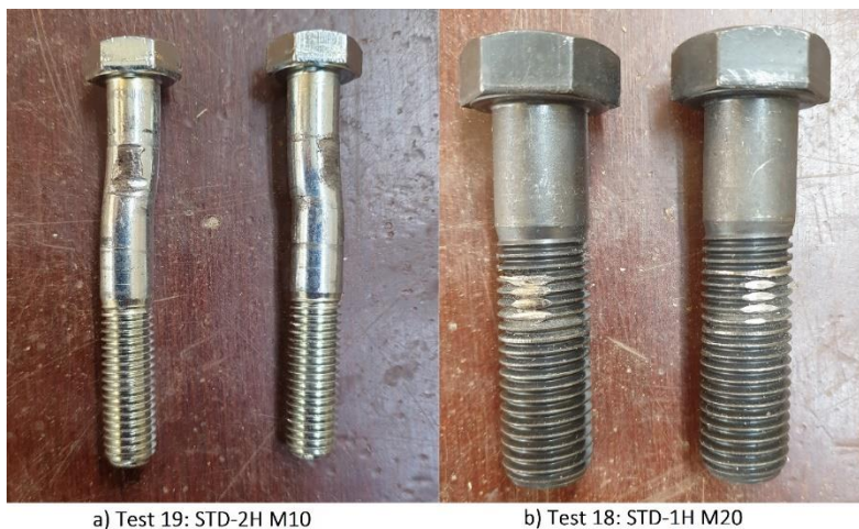
Figure 7-32 Damages to the bolts in a) test 19 and b) test 18
