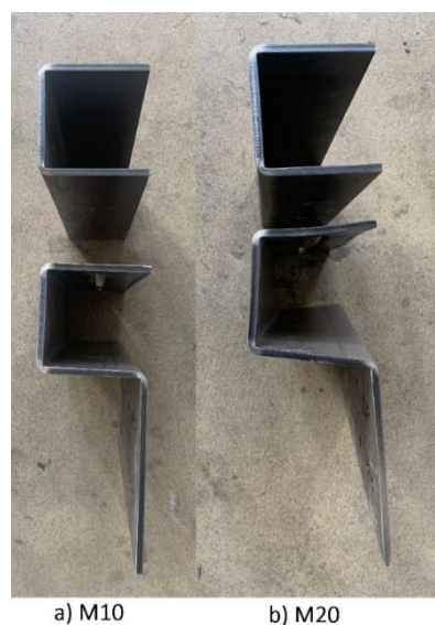
Figure 7-21 Twisting in a) STD-1H M10 and b) STD-1H M20
