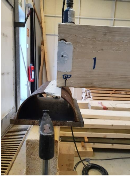
Figure 4.45 - Simply supported beam on steel rollers edgewise
