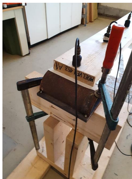
Figure 4.44 - Simply supported beam on steel rollers flatwise
