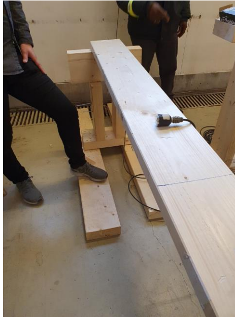
Figure 4.38 - Simply supported beam on timber supports
