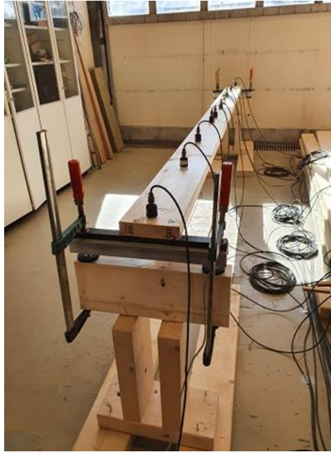
Figure 4.39 - Simply supported beam on rubber supports
