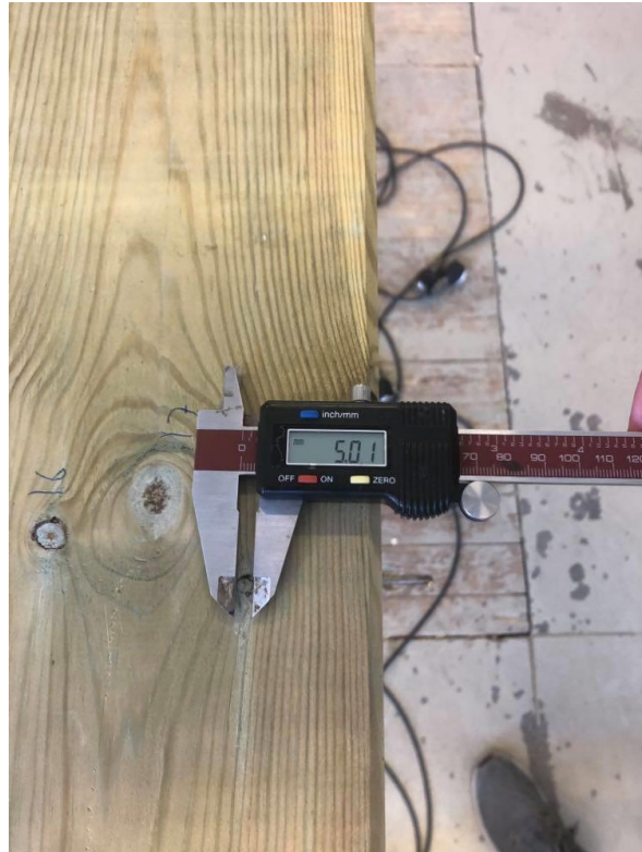
Figure 4.57 - Measurement of knot size
