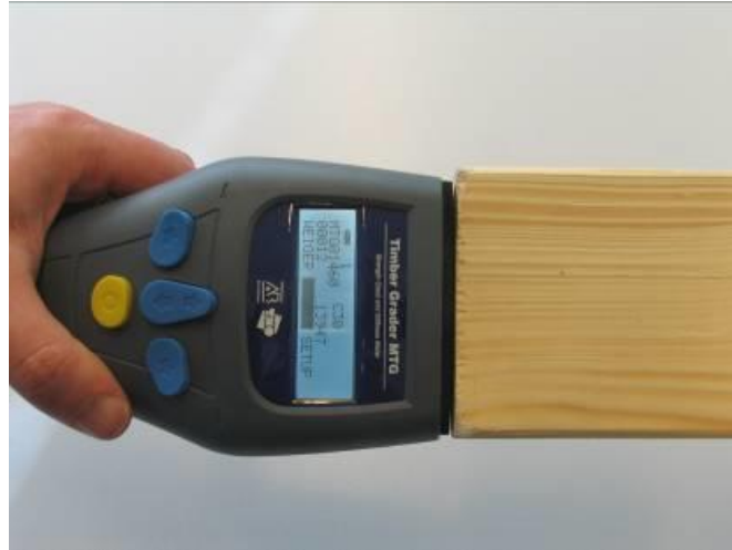
Figure 3.4 - How to use Timber Grader MTG
