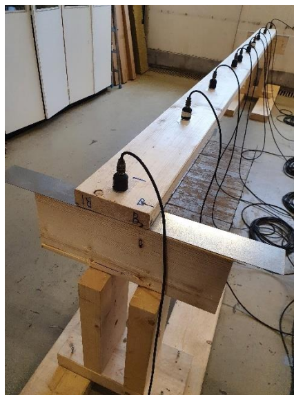
Figure 4.42 - Simply supported beam with steel plate
