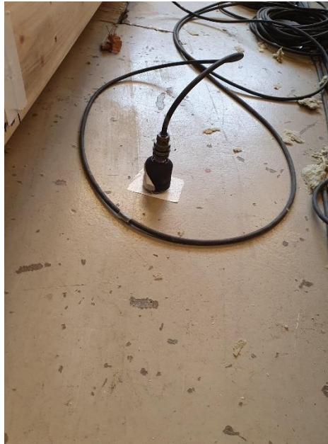
Figure 4.32 - Accelerometer on floor
