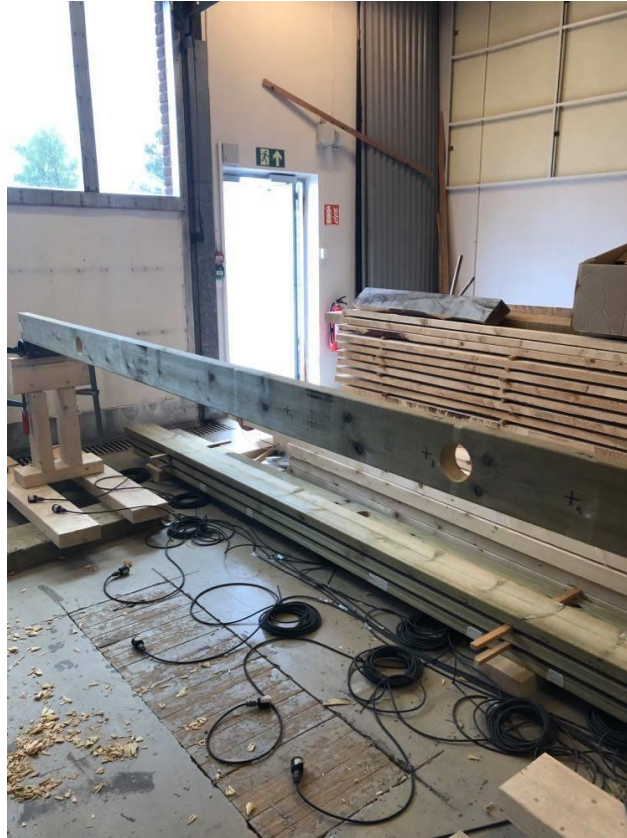
Figure 4.54 - Holes at quarter-points of beam
