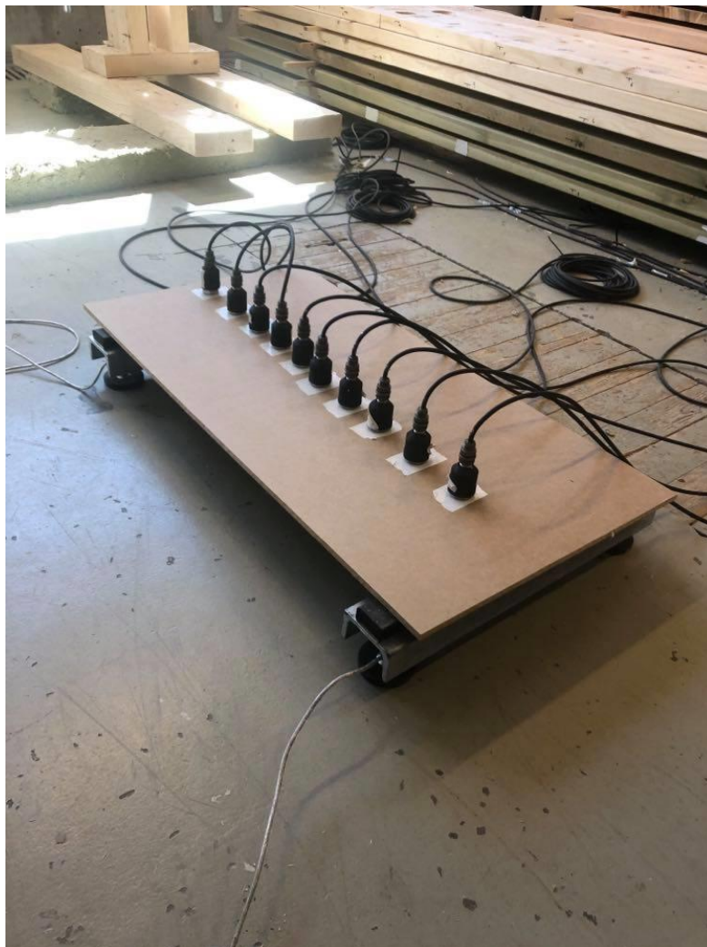
Figure 4.3 - Weighing of accelerometers
