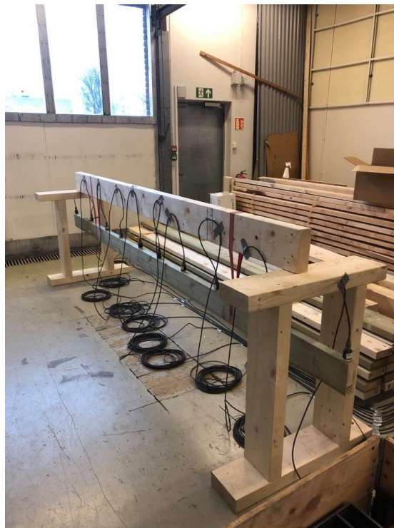
Figure 4.35 - Free-free support condition
