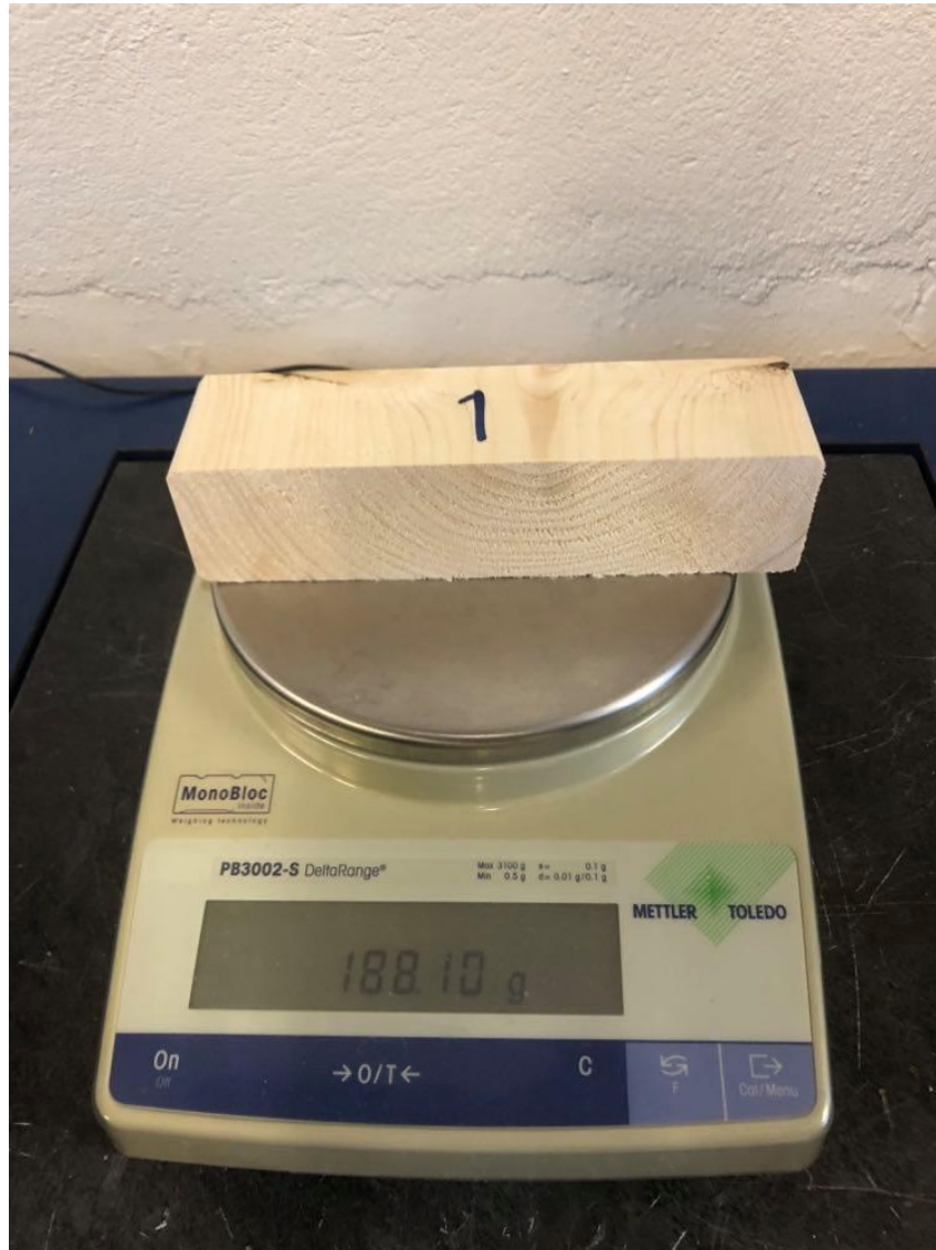
Figure 4.4 - Weighing of specimens with Bergmann PB3002-S Delta range scale
