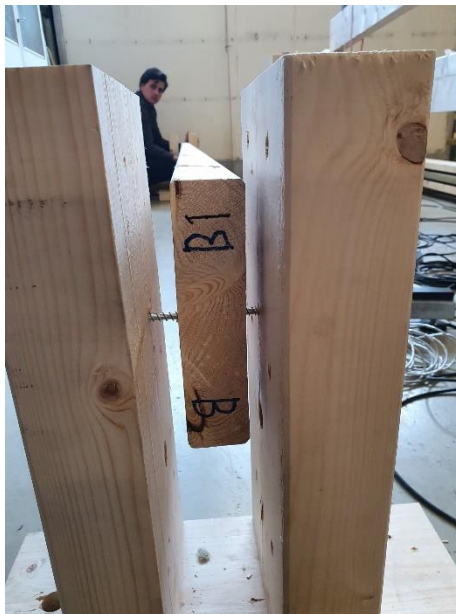
Figure 4.37 - Pinned-pinned support condition with screw
