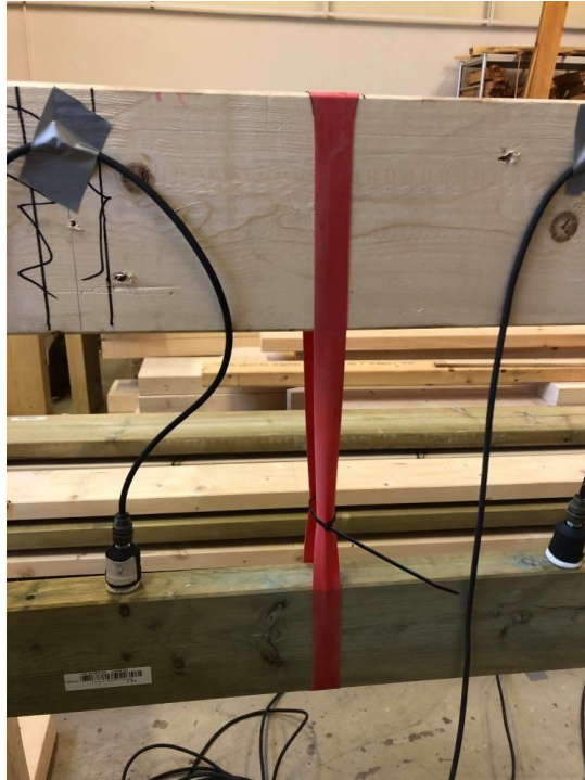
Figure 4.36 - Elastic bands as supports
