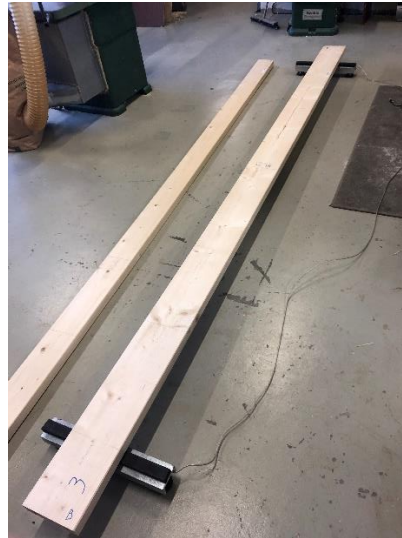
Figure 4.14 - Test setup for Timber Grader MTG
