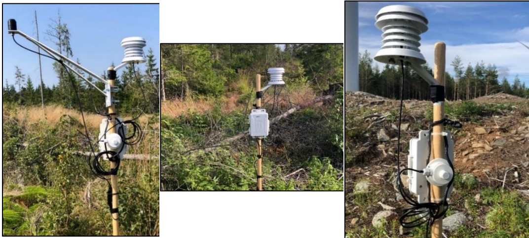
Figure 6. HOBOWare data logger set up between turbine & control site numbers eight and eleven.
