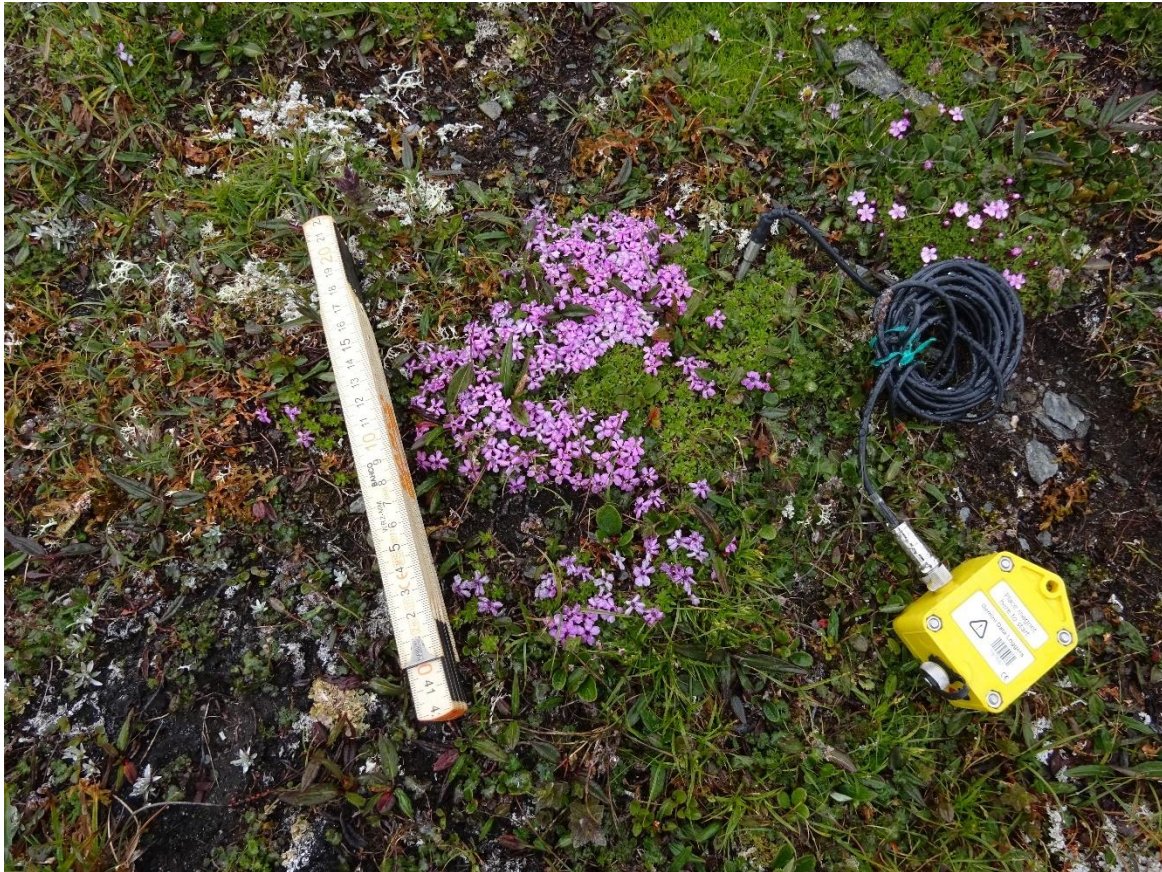
Figure 5: Tiny tag logger with a probe for soil temperature measurements placed next a S. acaulis cushion.
