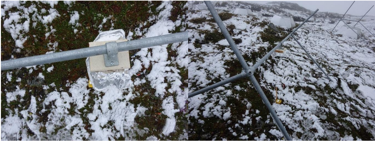
Figure 2: The cameras were mounted to a wooden plate and protected by an improvised housing of aluminum foil. The cameras were then mounted to a horizontal bar between a double A-frame. Five of these were placed at each site.
