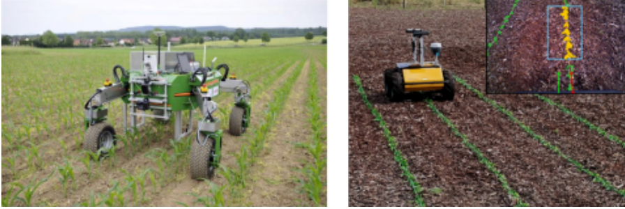
Figure 2.2: Example agricultural robot platforms with different navigation solutions. From top left: 3D row detection with BoniRob [Biber et al., 2012], vision-based (RGB) row detection in [Ahmadi et al., 2019].
