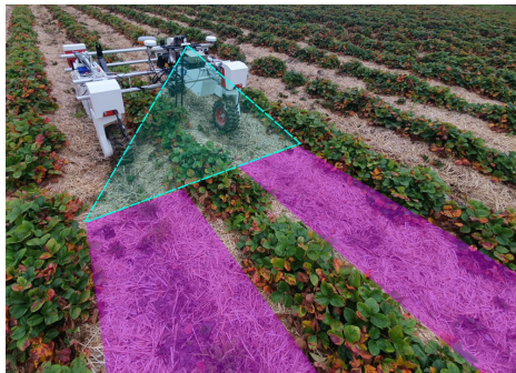
Fig. 1. The Thorvald II agri-robot platform operating in a strawberry field during data collection. We perform CNN-based segmentation to detect crop rows for visual guidance and propose an automatic labelling strategy for generating training data. During training, a mask representing crop locations is projected onto the camera image using the pose of the robot, measured with a dual-antenna RTK GNSS system. After training, CNN-based image segmentation can be used to guide the robot along the crop rows, without hand-drawn training labels.
