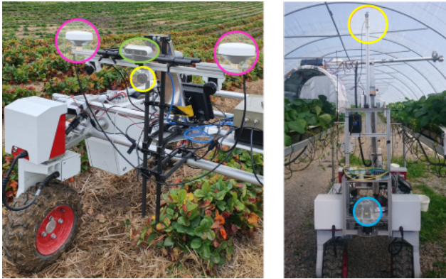
Figure 2.6: Robot setup for field data collection and experiments. Left: The Thorvald robot platform configured for a strawberry field, as used in Paper III and Paper V with RTK-GNSS antennas (pink), fisheye camera (yellow) and Intel RealSense D345 (depth was not used for this work). Right: The Thorvald robot platform configured for a strawberry polytunnel, as used in Paper I and Paper II with fisheye camera (red) and LIDAR laser scanner (blue).
