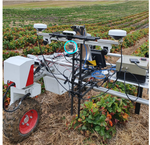
Figure 7: Data recording setup with robot in the field. The fisheye camera used for the recordings in this work is highlighted with a circle.
