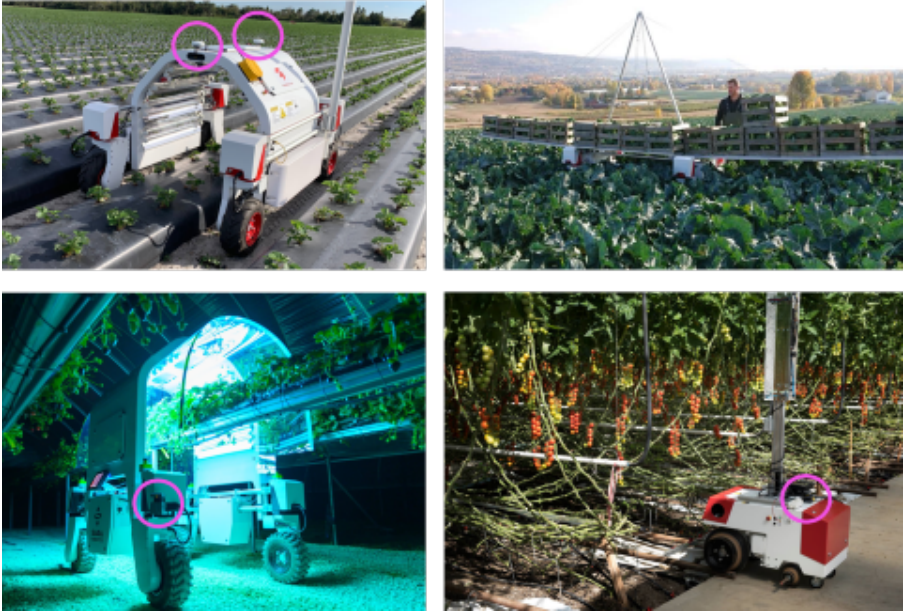
Figure 2.1: Example applications of the re-configurable Thorvald Robot platform. From top, row-wise: strawberries in field, broccoli in field, strawberries in polytunnel, tomatoes in greenhouse. Navigation sensors are highlighted with circles.
