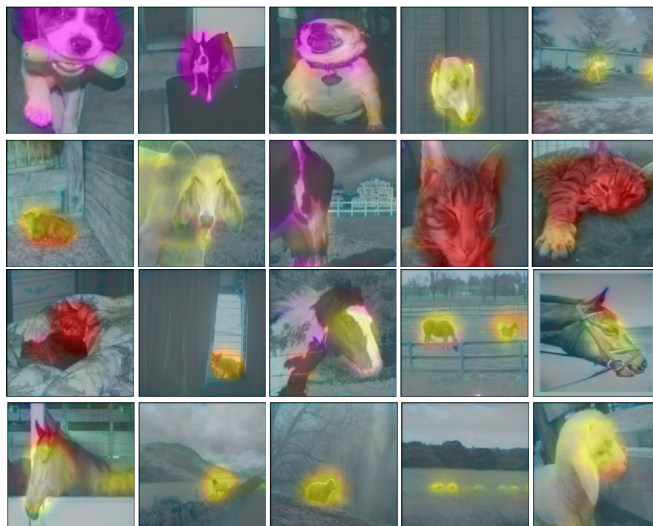
Fig. 7. Principal feature visualisation of VGG16 features on the Pascal VOC2012 dataset for the classes; “dog”, “cat”, “cow”, “horse” and “sheep”, with a batch of four random examples sampled from each class. Similar colours indicate similar features. Best viewed in colour.
