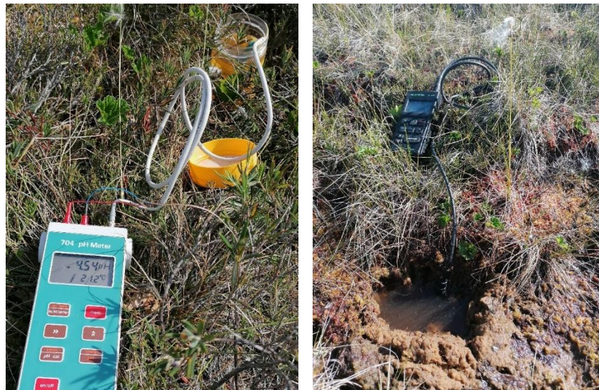
Figure 4. Left: pH was measured by first collecting water in a container, and then submersing the measuring cell of a pH meter into the container. Right: Electrical conductivity (EC) was measured by submersing the measuring cell of conductivity meter directly in the bog water.
