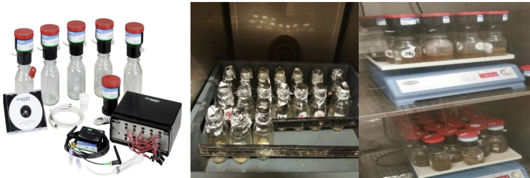
Fig. 4 Overall Ankom gas production operation procedure (Left: Ankom incubation bottles and modules, Middle: feed sample preparation before incubation, Right: feed incubation)
