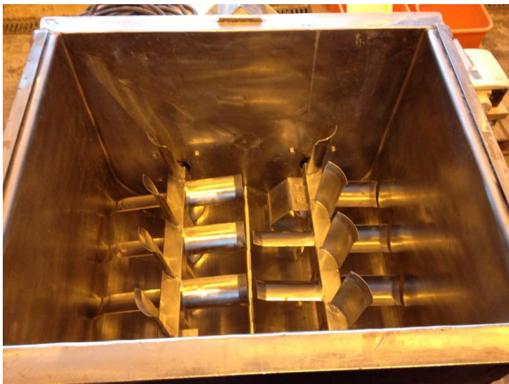
Figure 4. Idecon, 40 l, twin shaft paddle, self made mixer.
