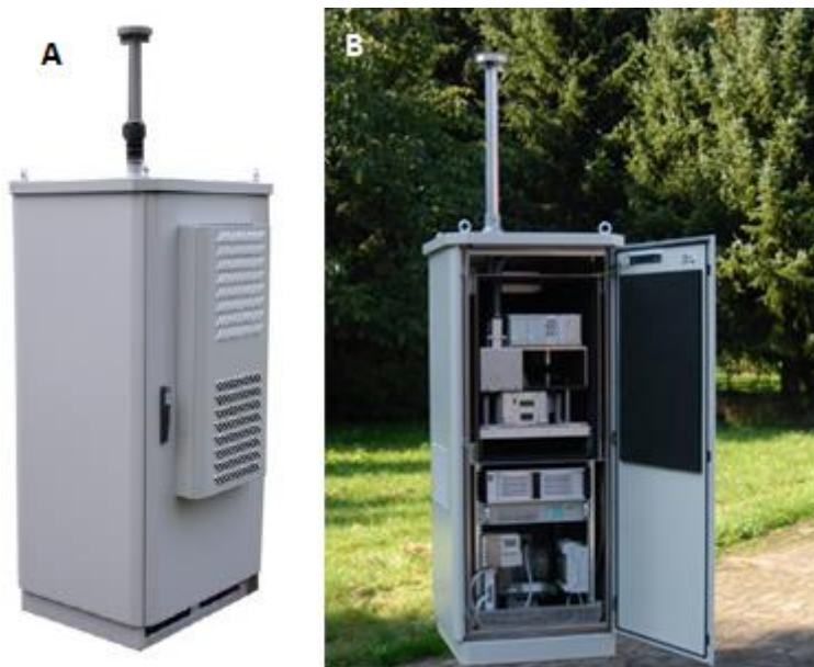
Figure 36: The pollen monitor BAA500. A: Exterior, from [55], B: Interior, from [56]
