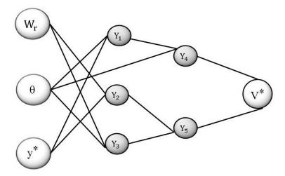
**Figure 7.** Evolved structure of generalized group method of data handling (GMDH) neural network for modeling and prediction of mean velocity.
