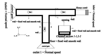
Figure 4. Boundary condition of the simulated model using the ANSYS-CFX.
