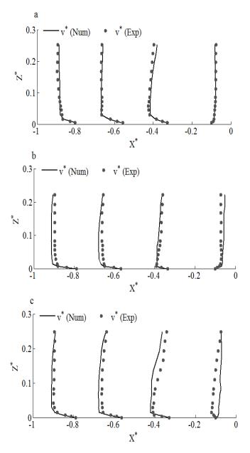
**Figure 5.** Verification graphs between the results of the CFX model and the Ramamurthy and his colleagues' experimental model in: (a)  $y^* = -0.29$ , (b)  $y^* = -1.00$ , and (c)  $y^* = -1.62$ .
