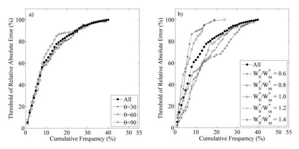
**Figure 9.** Error distribution of GMDH for (**a**) different angle ( $\theta$ ) (**b**) different relative width of branch channel to main channel ( $W_b^*/W_m^*$ ).
