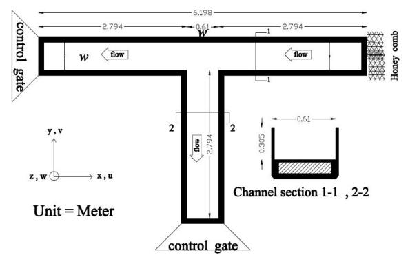
Figure 1. The plan of the experimental channel used in current research.
