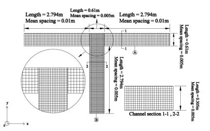
Figure 3. Gridding the plan and the cross-section of the simulated model using the ANSYS-CFX.
