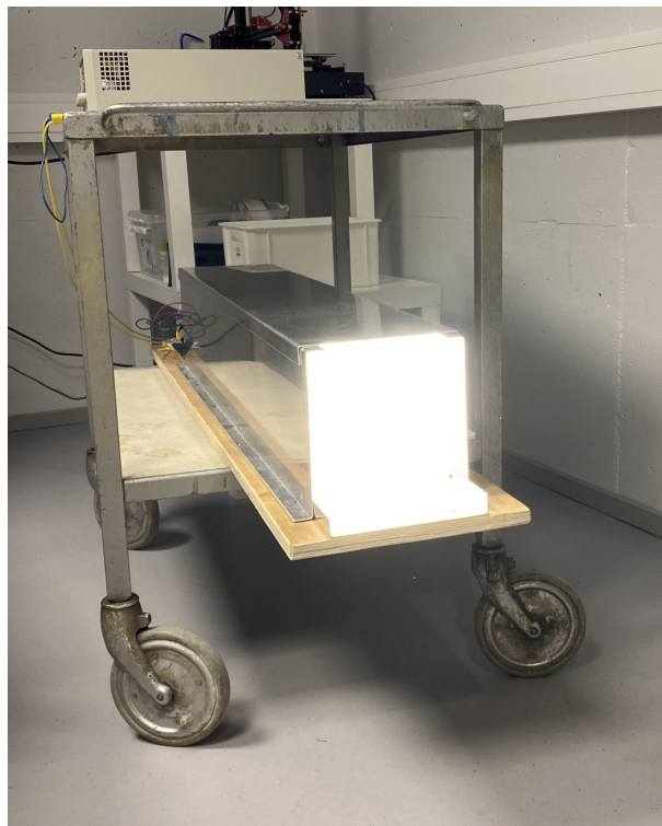
Figure 3.1.7: Image of the light "tunnel" used to calibrate the sensors.
