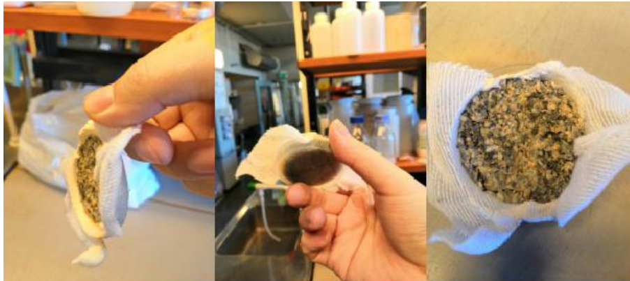
Figure 3. P-fertilizer disk for Soil Bypass Phosphorous (SBP disk). The rock sand with Ca (H 2 PO 4 ) 2 is placed in a 5 cm diameter petridish lined with gauze, which is then flooded with molten agar. Once the agar is solidified, the disk is airdried, and ready to use. Upon rewetting, the agar swells to 30% of the original volume, securing ~70% air filled macropores.
