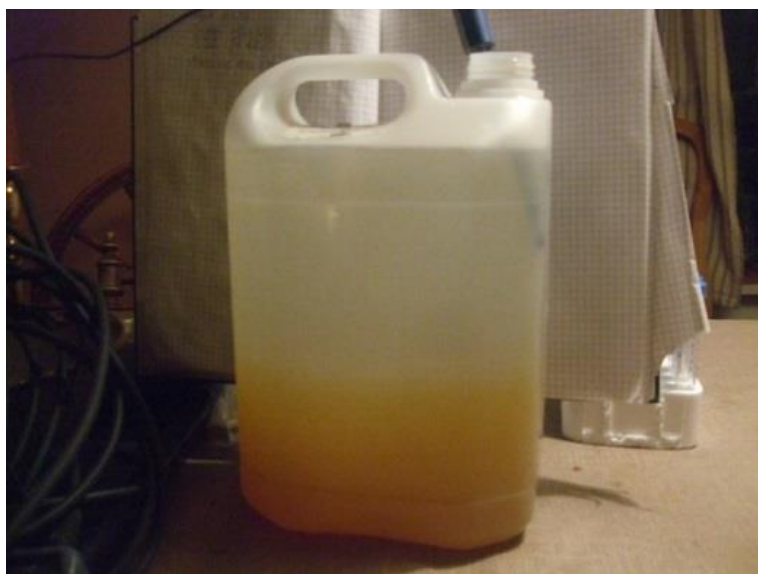
Figure 18: Precipitation after addition of NaOH in 5 L plastic can with sample water (AMD) from Site 2.
