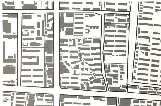
Figure 3. Example of modernist urban tissue with different patterns of freestanding buildings in open spaces (image by Kropf, 2018, p. 46)
