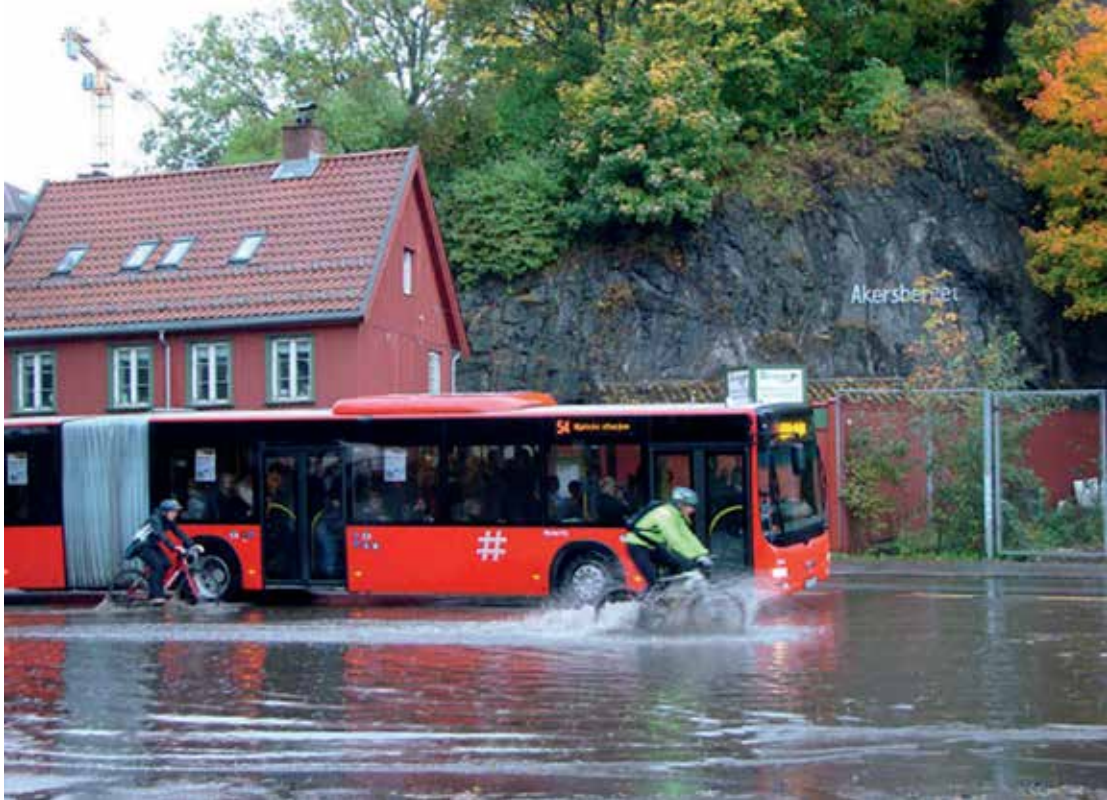
Photo 3.1 Oslo is no stranger to urban flooding due to stormwater runoff traveling rapidly along impermeable surface, seen here outside Oslo's school of Architecture and Design (AHO). The city's sloping terrain further accelerates the water's velocity (p. 5). Photo by Hanne Johnsrud.
