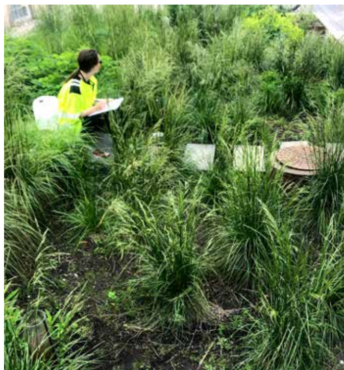
Photo 6.2 MPD infiltration testing in rain garden 1
