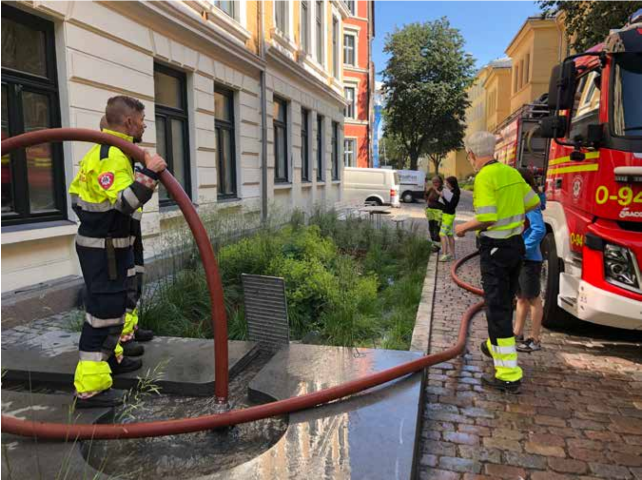
Photo 6.10.a Simulating heavier rainfalls in rain garden 7, with the help of Oslo's fire department.
