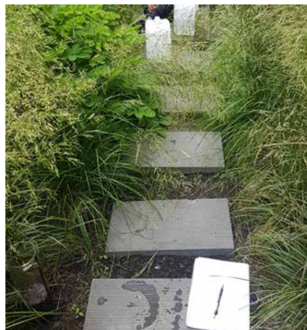
Photo 6.4 MPD-testing in rain garden number 4, the test tube is visible in the bottom left corner of the photo.
