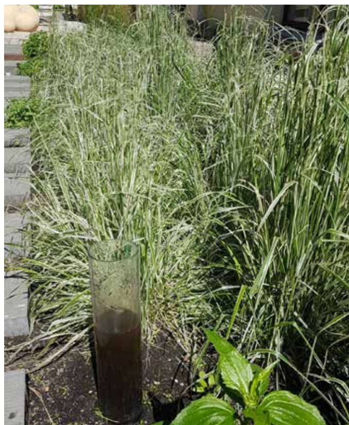
Photo 6.9 MPD-testing in rain garden 9. Pouring the water too quickly can cause soil particles to mix with the water, as seen in the photo.
