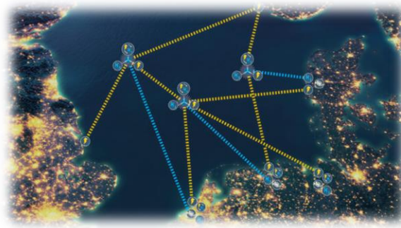
Figure 30 Vision for North Sea Wind Power Hub. Offshore wind farms in North Sea are connected to artificial hub islands, enabling multi country connection points for electricity transmission through HVDC stations (yellow lines) and production of hydrogen from excess power which can be transported through pipes (blue lines). Source: North Sea Wind Power Hub. (2019). Retrieved 3/11, 2020, from https://northseawindpowerhub.eu/key-players-wind-industry-support-ex-amination-feasibility-of-north-sea-wind-power-hub/ .
