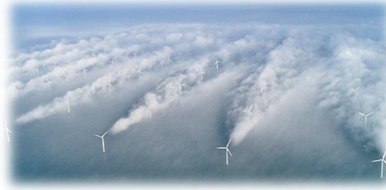
Figure 17 Real-life photography of wake effect at Vattenfall's Horns Rev 1 wind farm. Source: Fialka, J. (2017, December 11). 'Wake' mystery is mostly fixed, helping turbines best coal. Retrieved from E&E News: https://www.eenews.net/stories/1060068565
