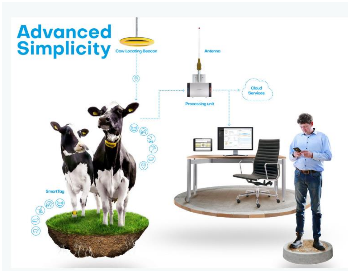
Figure 1. Illustration of Nedap, where the cow on the left is wearing a Smarttag Leg and the cow on the right is wearing a Smarttag Neck. Registration at cow level is uploaded to an internet cloud, from which the data can be viewed and downloaded. (Nedap Livestock Management, n.d.)
