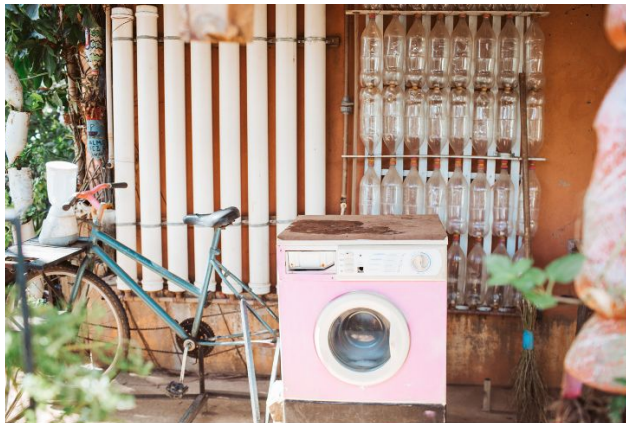
← Bicycled powered blender and washing machine connected to plastic bottle rainwater catchment system
