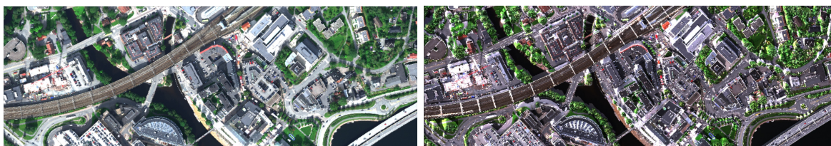
Figure 2.6: Left: Radiance Image, Right: Reflectance Image. Both images are of the same place but the radiance and reflectance image looks different. The radiance image is a bit brighter and clear as compared to the reflectance image. Some of the parts of the radiance image are overexposed, whereas the reflectance image is well exposed.
