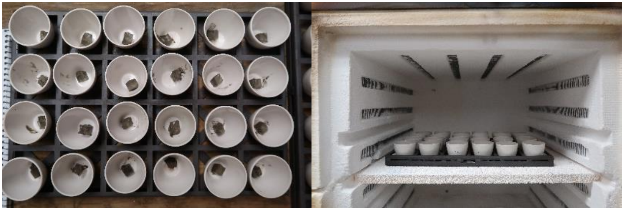
Figure 4.4: Left: The sediment collected every 1cm was placed in a crucible. Right: The sediment samples in the crucible were placed in a drying oven.
