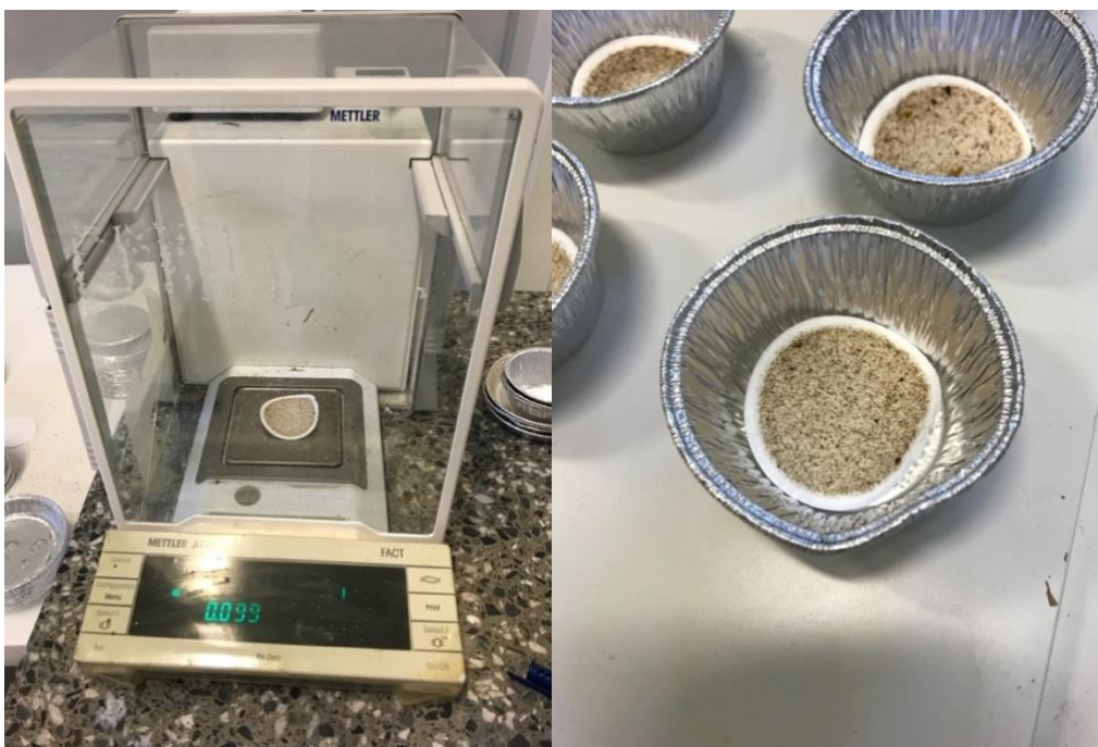
Figure 4-7: Weighing the filter and suspended solids after drying
