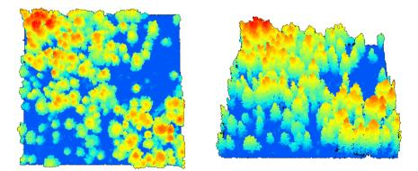
Fig. 2. Example of an airborne laser scanning point cloud seen from above (left) and from a top side view (right). Colors indicate the height of laser echoes, ranging from low values (blue) to high values (red).
