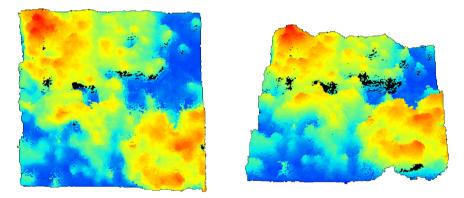
Fig. 3. Example of a digital aerial photogrammetry (DAP) point cloud seen from above (left) and from a top side view (right). Colors indicate point heights ranging from low values (blue) to high values (red). As opposed to airborne laser scanning data (Fig. 2), DAP data mainly characterize the outer envelope of the canopy; gaps within the canopy are less well defined, and sub-canopy vegetation and terrain surface are poorly characterized.
