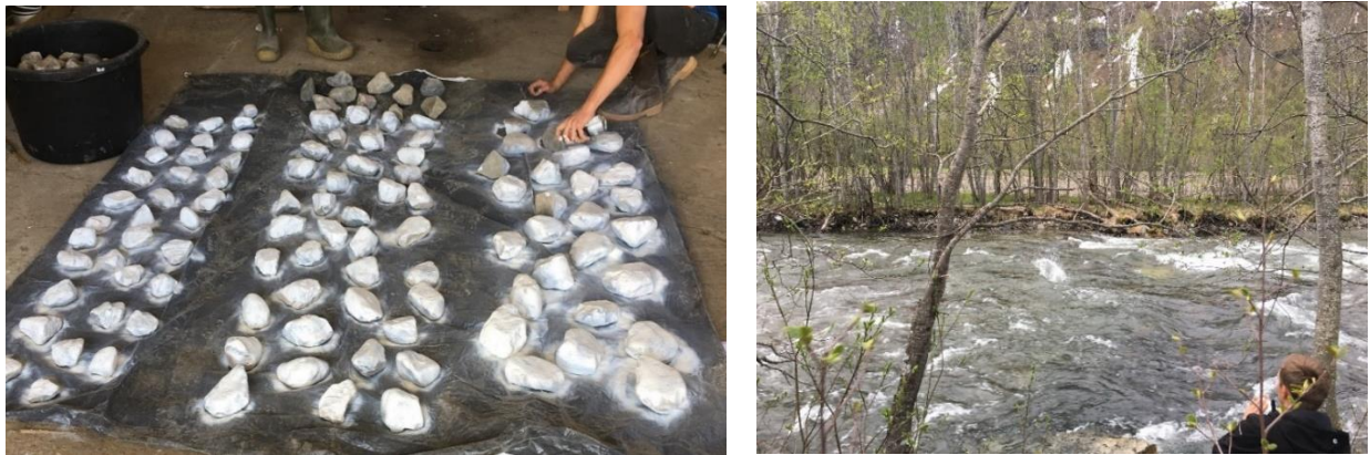
Figure 3. Left: Photograph of painted white rocks that have an inserted pit-tag, and divided into rows of each of three weight classes. Right: Releasing of rocks in field. Picture is taken at station 5.
